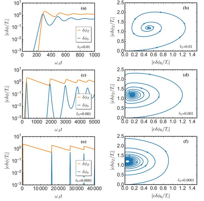
FIG. 2. (a), (c), (e): TAE  $\delta\phi_0$  and zonal potential  $\delta\phi_Z$  evolve to the fixed points in: (b), (d), (f). ZM collisional damping rate  $\hat{\nu}_{ii} \equiv \nu_{ii}/(\hat{\chi}_{iZ}\omega_A)$  is decreased from top to bottom.  $\gamma_1$ ,  $\gamma_2$  and  $\gamma_d$  are the same as in Figure 3.
