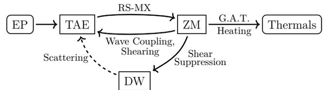
FIG. 1. A feedback diagram for TAE and ZM with energy deposition from EP to thermals. ZM saturates TAE and suppresses DW turbulence. Thermal plasma damps ZM and so is heated.
