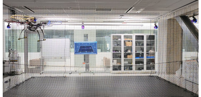
Fig. 6. Experimental setup for indoor flight testing at the Flight Dynamics and Control Lab, GWU. A custom-designed quadrotor UAV, developed for sim-to-real transfer, is tracked by a 12-camera Vicon Valkyrie VK-8 motion capture system. Position and attitude measurements are transmitted to the onboard NVIDIA Jetson TX2 at 200 Hz via Wi-Fi.
