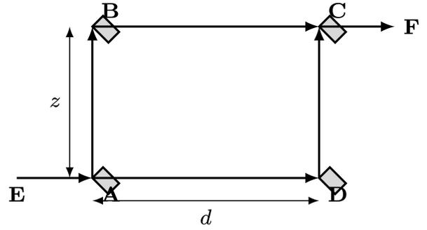
Figure 1. Schematic diagram of a neutron interferometer. The incoming beam (E) is split by mirrors at points A, B, C, and D, and recombined into the outgoing beam (F). The enclosed area is given by  $A = z d$ .
