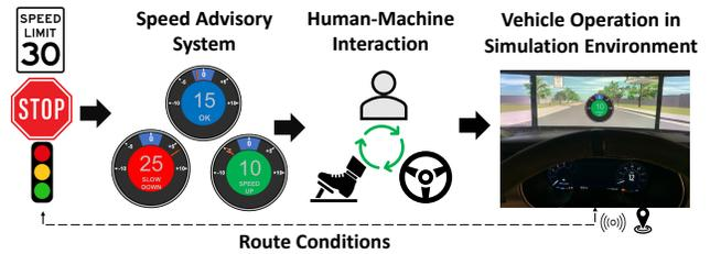
Fig. 1. Speed advisory system in the driver-in-the-loop simulator.
