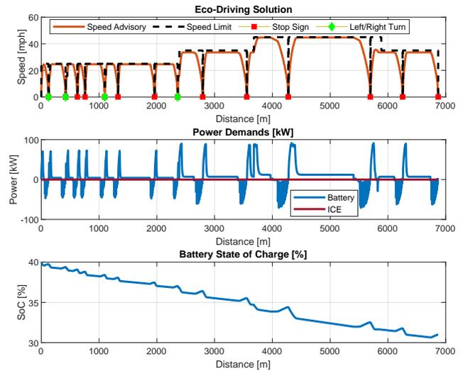
Fig. 2. Speed profiles, power demands, and battery state of charge profiles provided by the optimal solution in the speed advisory system.
