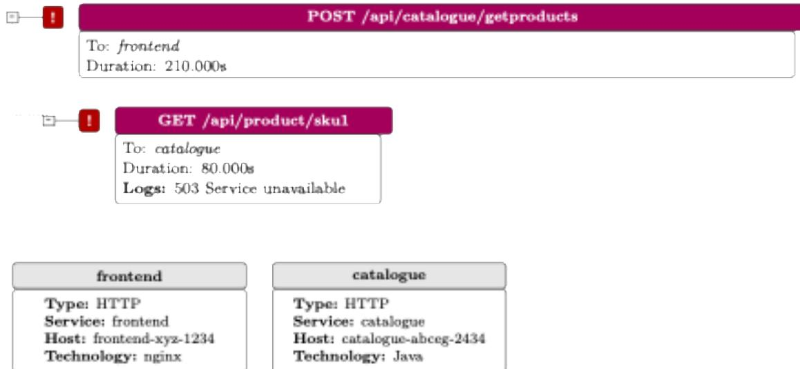
Figure 2. Trace of a failed request from frontend to the catalogue service
