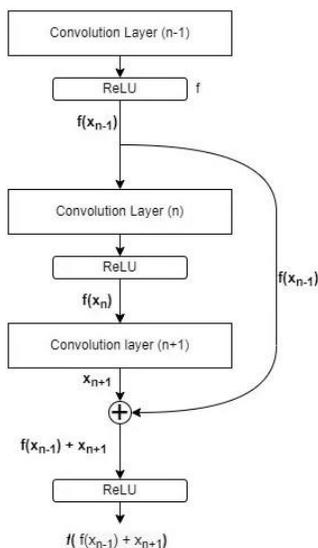
**Figure 8:** A skip connection within ResNet
