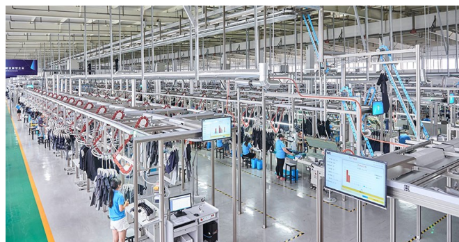
Fig 2 Intelligent Hanger Line and System from INA Intelligent Technology (Zhejiang)
