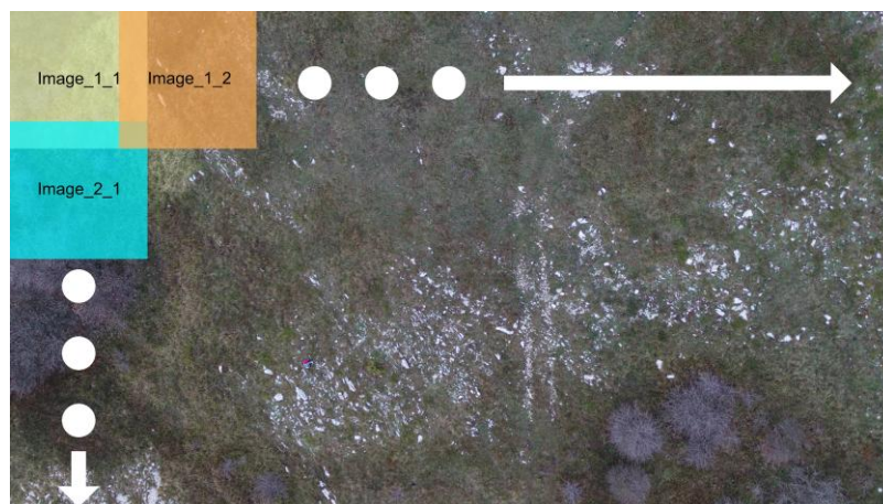
Figure 2 The tiling method used to divide original sized images into images of 512 \times 512 pixels. The overlap ensures more context being available in the newly created dataset.
