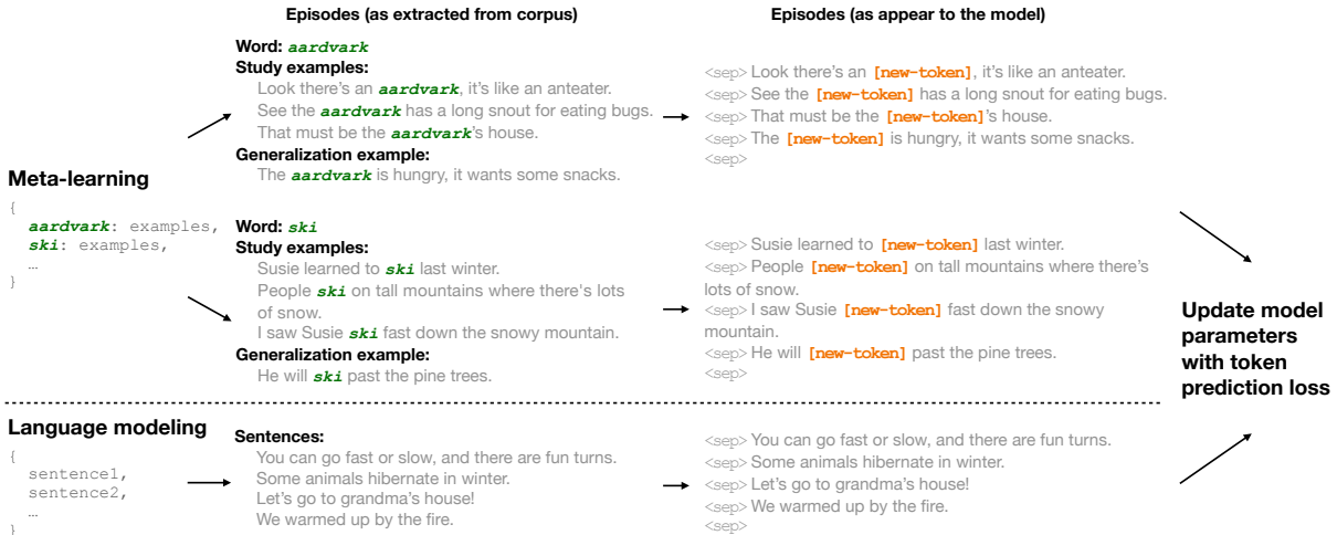
Figure 1: Illustration of Minnow (top) and language modeling (bottom), which can be mixed together during training such that both contribute to model updates. Each meta-learning episode in Minnow aims to learn a new word from a set of study examples (sentences that use the word) in the context and then generate a generalization example that also uses the word. Each language modeling episode contains a set of unrelated sentences without meta-learned words. An episode will be converted into a single sequence in which we replace the word to be learned (if it is a meta-learning episode) with a special placeholder token (e.g., [new-token] ) and concatenate/wrap the sentences with another special separator token (e.g., <sep> ). We do gradient updates of the model parameters to optimize the next-token prediction loss on the sequence.
