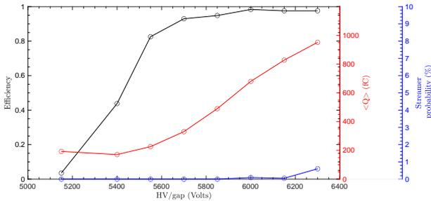
Figure 3: Response of the sRPC to atmospheric muons before bunker irradiation as a function of the voltage applied in each gap showing an efficiency plateau of around 98% above 6000 V.
