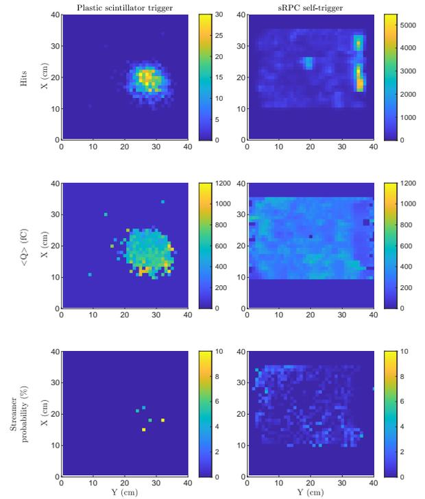
Figure 4: Response of the sRPC before bunker irradiation as a function of the 2D position. a) b) and c) correspond to atmospheric muons and d), e) and f) to self-trigger.
