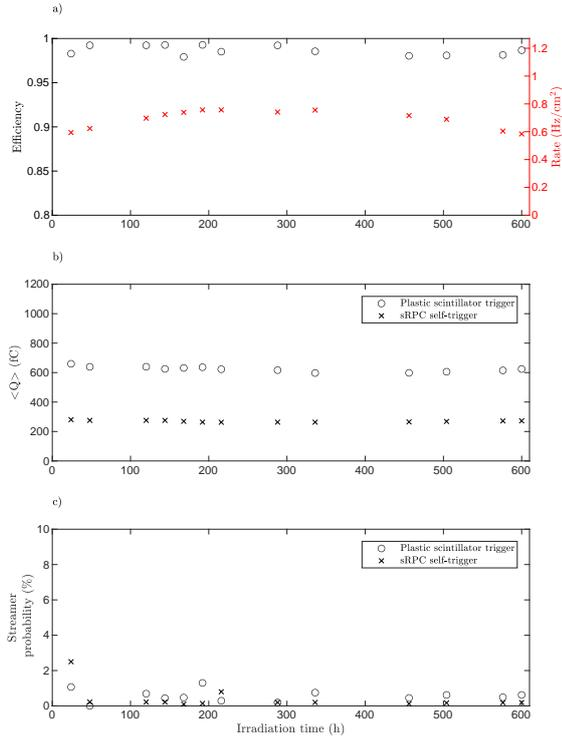
Figure 5: Response of the sRPC to atmospheric muons during the irradiation period of approximately 600 hours with the cobalt source. The analysis includes efficiency, background rate, average charge and streamer probability. Each point corresponds to approximately two hours of data collection without the cobalt source, after twenty two hours of exposure.
