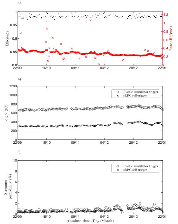
Figure 6: Response of the sRPC to atmospheric muons during four months in the laboratory after bunker irradiation. The analysis includes efficiency, background rate, average load and streamer probability.
