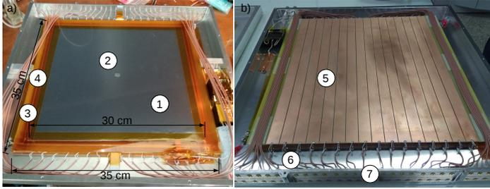
Figure 1: a) sRPC module showing: 1- HV layer, 2- Circular spacer in the center of the active area, 3- Strip spacer all around the periphery and 4- Mylar™ and Kapton™ layers. b) sRPC plane showing: 5- Readout strip plane, 6- Coaxial cables and 7- MMCX RF feedthrough connectors.
