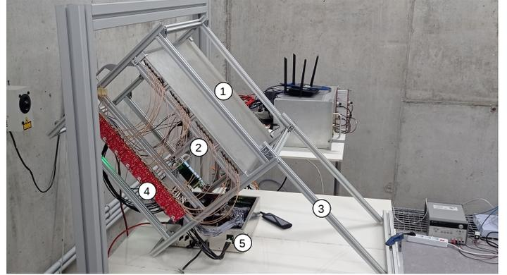
Figure 2: Bunker arrangement: 1- sRPC, 2- location of the mini-telescope based on four plastic scintillators (not visible on the picture), 3- aluminum structure, 4- FEE and 5- DAQ box containing the TDC board and a single board computer together with the necessary ancillary elements.
