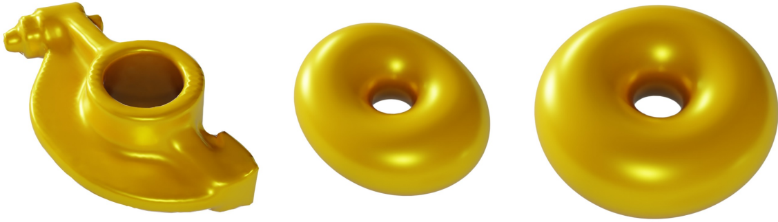
Figure 7: Evolution of a rocker arm shape under Willmore flow. The spatial resolution is n = 64 , the kernel size is n_K = 17 , the interface parameter \varepsilon = 2^{-5} , the inner MCF stepsize \tilde{\tau} = 2^{-12} , and the Willmore flow stepsize \tau = 2^{-12} . We show the discrete timesteps 0, 1, and 20 leading to an approximation of the Clifford torus.
