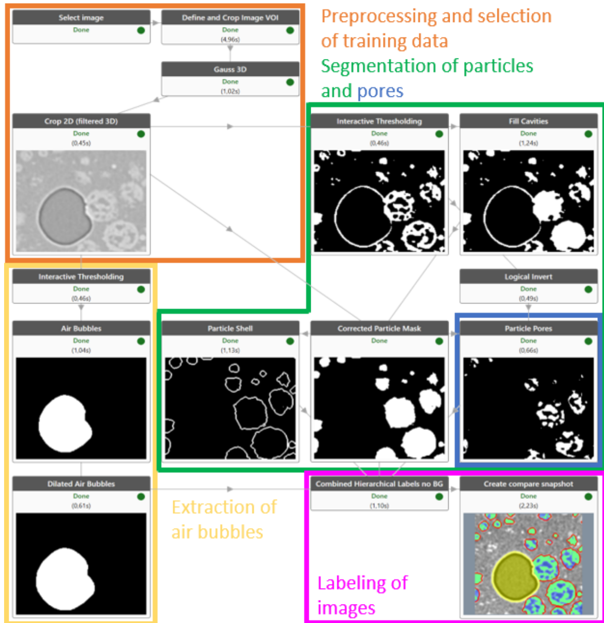
Figure S8: First workflow step (1) of the XamFlow analysis, the generation of the 2D training data for the Unet segmentation. It can be split into four sections: The preprocessing and selection of training data, the segmentation of particles and pores, the extraction of air bubbles and finally the labeling of the images.
