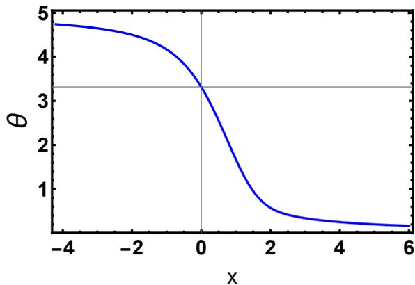
FIG. 2. The average blowup time  $\Theta(x)$  versus the initial position  $x$  for  $n = 2$ , see Eq. (18). Here  $\Theta(-\infty)/\Theta(0) = 3/2$ , as predicted by Eq. (20).
