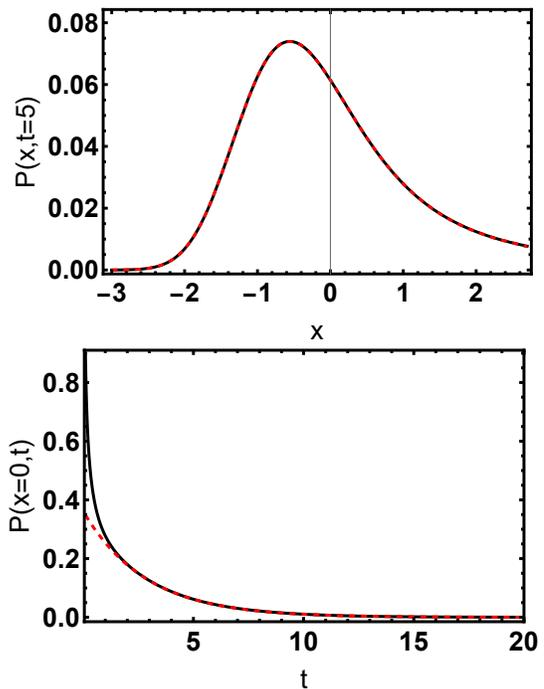
FIG. 10. The position distribution  $P(x, t)$ , computed numerically for  $n = 2$  (solid lines). Dashed lines: predictions from the single-mode long-time asymptotic (43).
