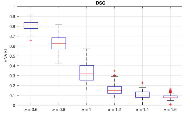
Figure 21: Boxplot of the ENVSI indicator calculated based on Monte Carlo simulation for 100 iterations of the cyclic component (Class 2) for several levels of the noise (expressed as  $\sigma$ ).
