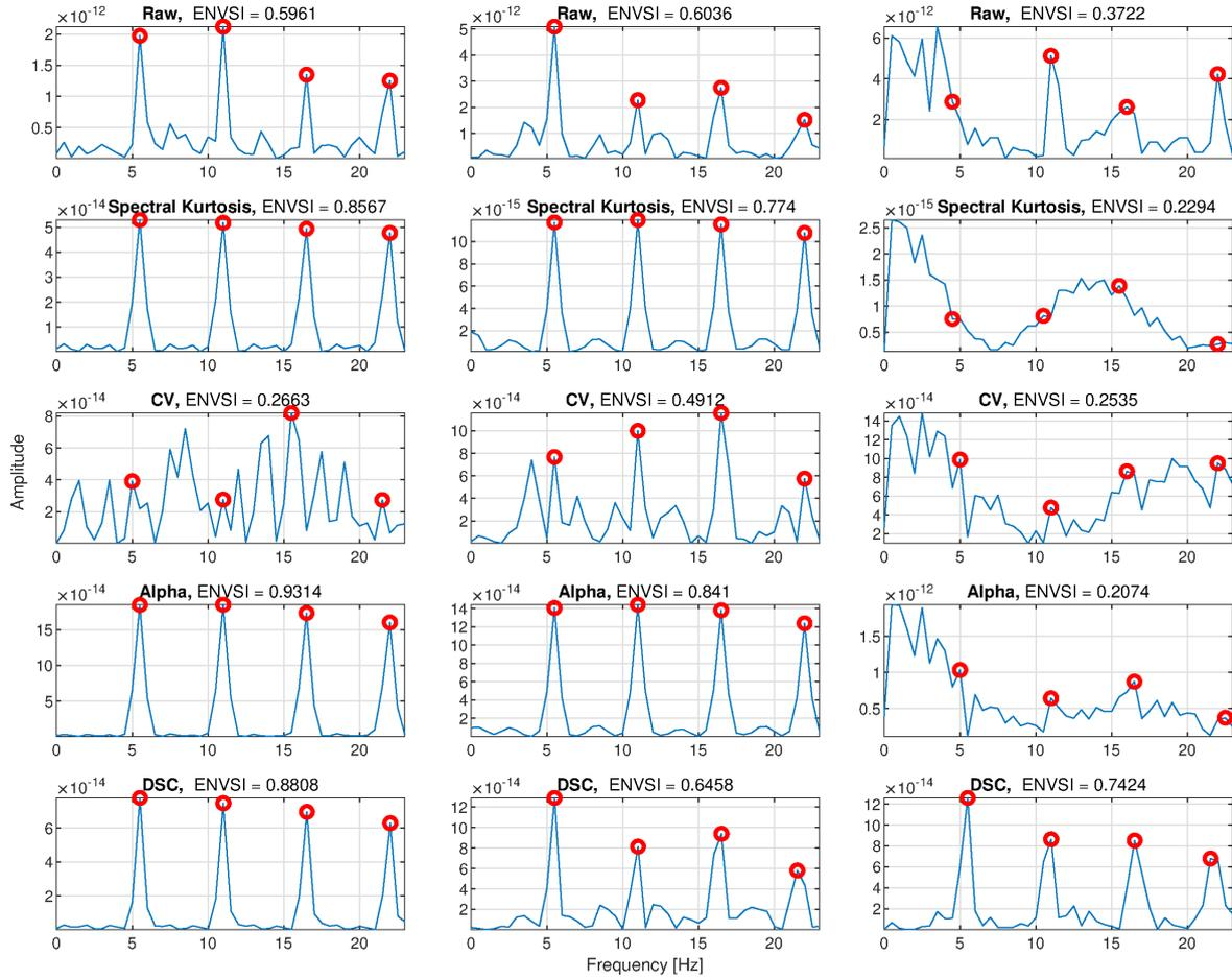
Figure 19: The squared envelope spectra for the raw signal and all compared method.
