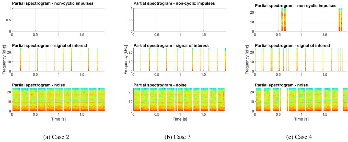
Figure 17: Visual representation of DBSCAN clustering of the real acoustic data.
