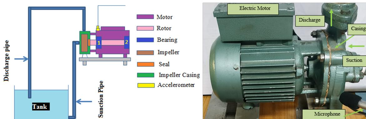
Figure 10: The scheme (left panel) and the photo during the acoustic measurement session (right panel) of the test rig.
