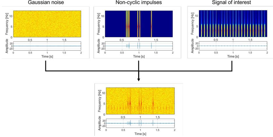
Figure 2: Construction of the analyzed signal.
