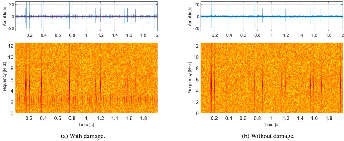
Figure 6: Time series of simulated signal for  $\sigma = 0.6$  and  $\gamma = 3$  with corresponding spectrogram. Left panel with added SOI component of  $f_{mod} = 30.7$  Hz and right panel without damage.
