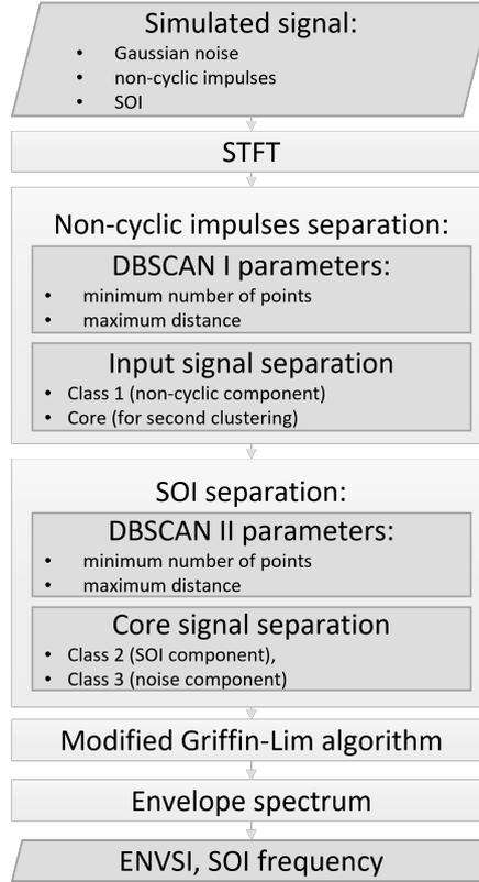
Figure 1: Flowchart of the proposed procedure.
