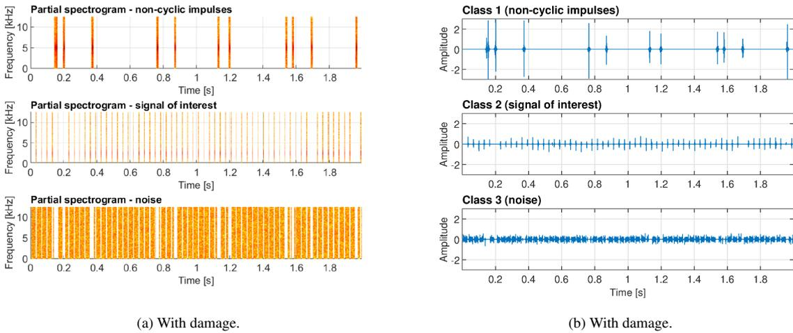
Figure 7: Partial spectrograms divided by classes 1-3 with related time series for a signal with SOI component.
