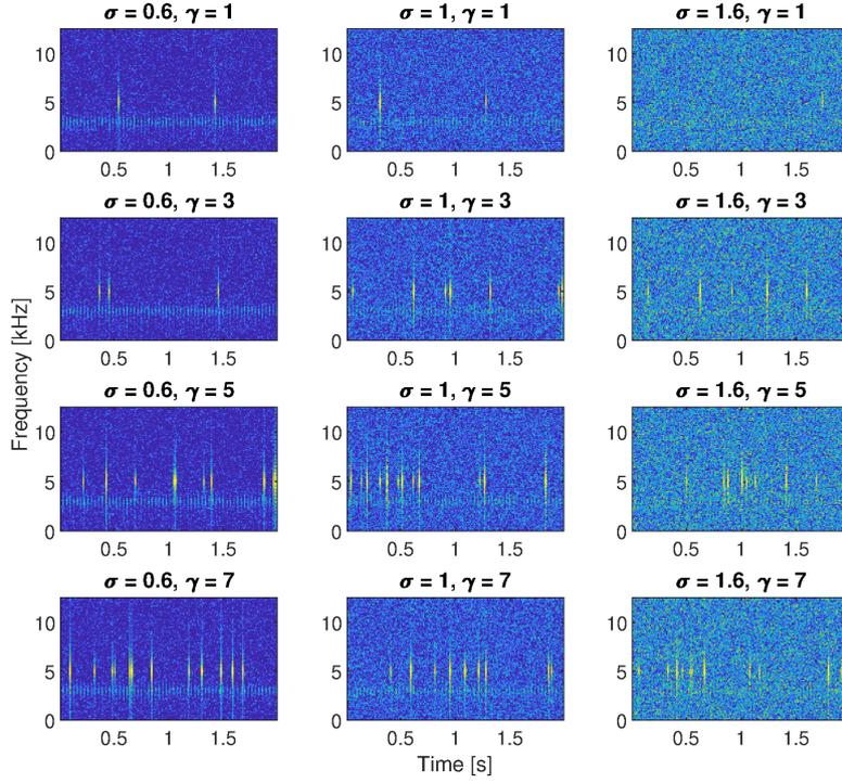
Figure 5: Spectrograms of the exemplary simulated signals for fault frequency  $f_{mod} = 30.7$  Hz.
