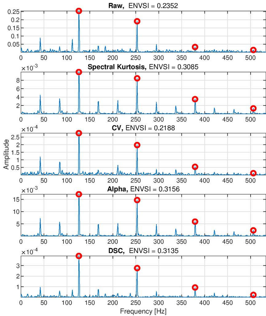
Figure 14: The squared envelope spectra for the raw signal and all compared method.
