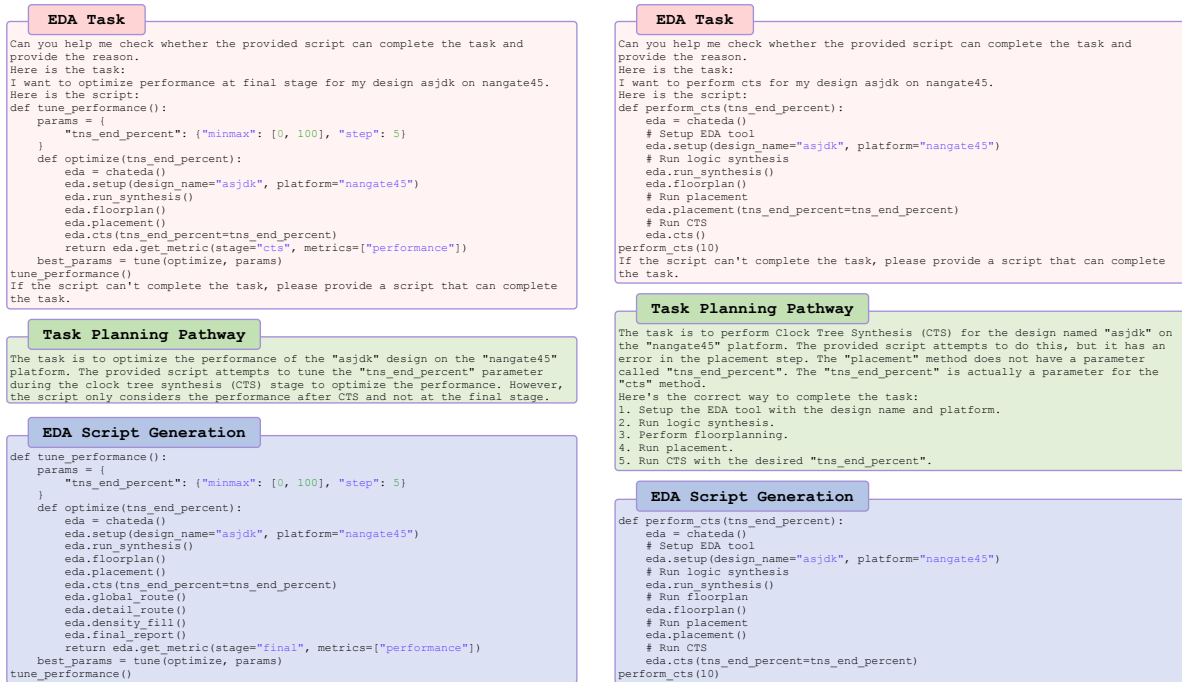
Figure 7: Error correctness. The decision-making agent (role R_1 ) can identify and fix errors in given EDA scripts accurately according to the given EDA tasks.
