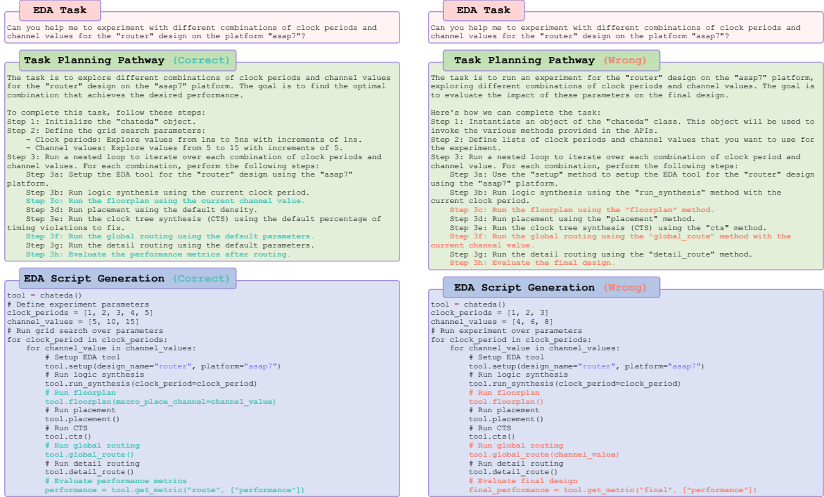
Figure 6: Divergent thoughts. Right: the divergent-thoughts agent (role R_0 ) generates correct task planning pathways and EDA script. Left: the divergent-thoughts agent (role R_0 ) makes mistakes in intermediate steps.
