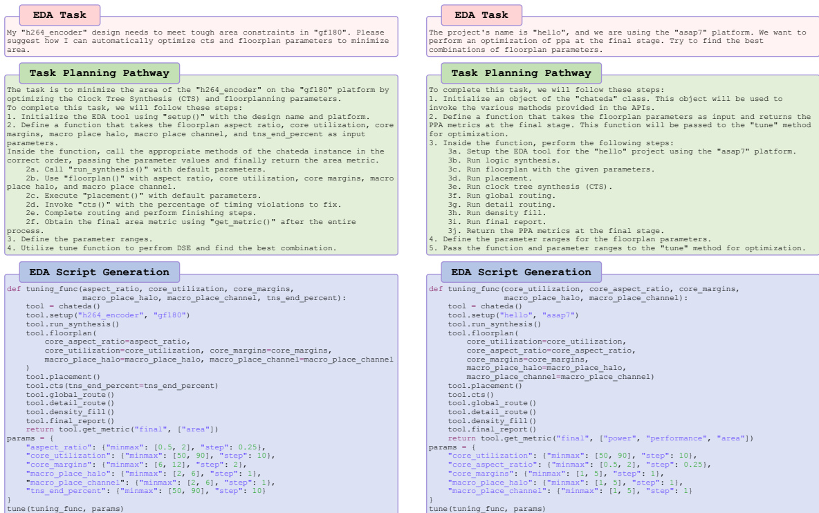
Figure 8: Case Studies of EDA flow automation with our EDAid powered by ChipLlama models. Each case provides an EDA task, its corresponding task planning pathway and the generated EDA script.
