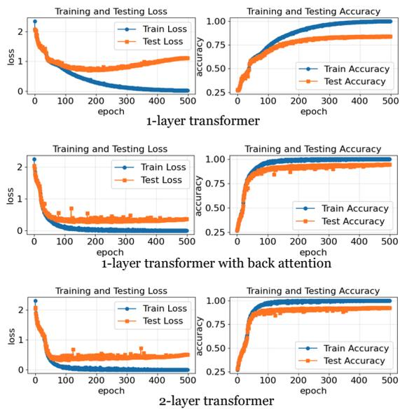
Figure 16: Loss (left) and accuracy (right) on arithmetic dataset of 1-layer transformer, 1-layer transformer with back attention, and 2-layer transformer.
