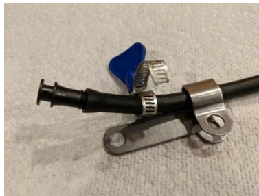
Figure 9. Use of worm gear clamps facilitated easy setup and removal of the tube system.
