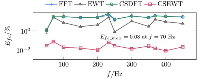
Fig. 8.  $E_{fc}$  of four algorithms under harmonic disappearance.
