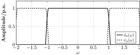
Fig. 4. The transfer function of EWT ( $\gamma = 0.01$ ).
