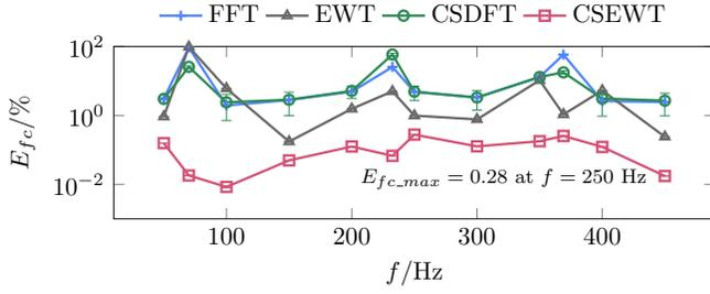
Fig. 7.  $E_{fc}$  of four algorithms under amplitude swell.
