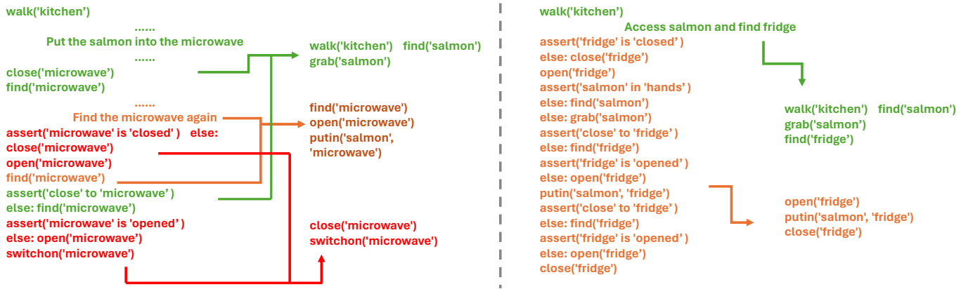
Fig. 3. Qualitative analysis. The two planning examples, “Microwave Salmon” (left) and “Put Salmon In The Fridge” (right), show the comparison between two plans generated by Prog-Prompt [17] (on the left of each side) and our method (on the right of each side). Commands in red represent what Prog-Prompt did wrong and redundantly, while our method did correctly and concisely. Commands in orange represent what Prog-Prompt did redundantly while our method did concisely. Commands in green represent necessary and correct commands for both Prog-Prompt and our method.
