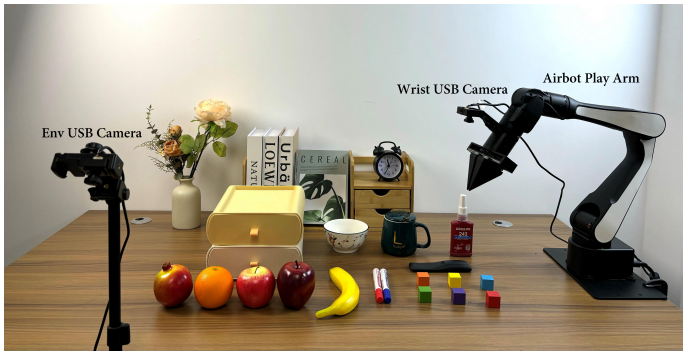
Fig. 4: Our robot setup and everyday objects. We use Airbot Play 6-DoF robot arms including a gripper and a teacher to demonstrate and inference. We also employ diverse everyday objects for our manipulation tasks and visual distraction. Two USB cameras are used to capture global and wrist view visual observations.
