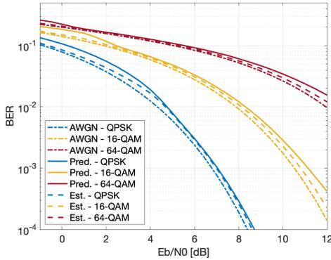
Fig. 3. BER as a function of  $E_b/N_0$  (NTN-TDL-C).
