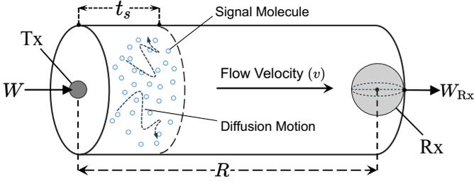
Fig. 1. Molecular propagation channel with a point Tx and a spherical Rx.
