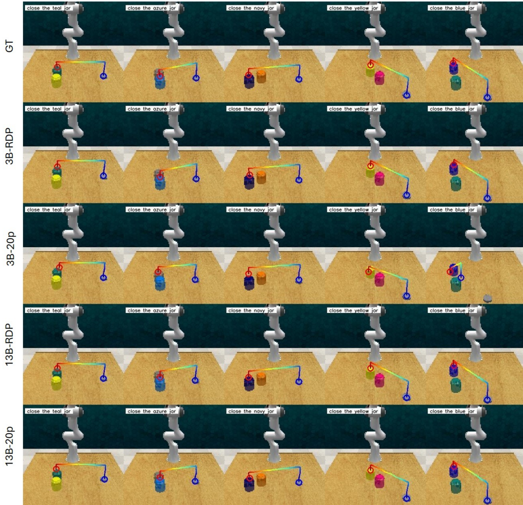
Figure 17: The task is to pick up the lid and close it on the jar with correct color. Task description is located on the top-left corner of each image. The trajectory goes from blue to red where blue circles denotes where the gripper should close and red circles denotes where the gripper should open. GT denotes ground truth, 3B and 13B denotes VILA1.5-3B and VILA1.5-13B, RDP denotes paths simplified using Ramer–Douglas–Peucker algorithm while 20p denotes paths represented using 20 points.
