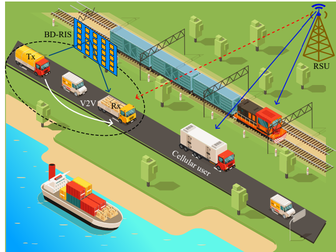
Fig. 3: BD-RIS assisted V2V communication underlay cellular network.
