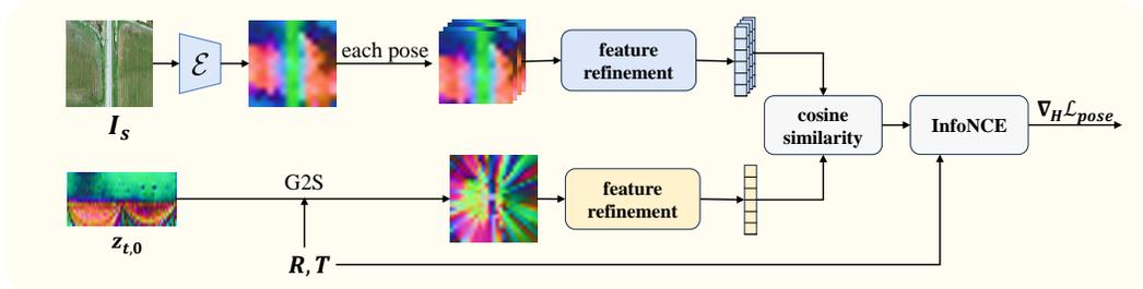
Figure 3: Homography Adjustment. We compare ground-level images with satellite images, calculating the loss by assessing the relative pose of the ground images at time  $t$  against a predefined pose. Ground images are then adjusted based on this comparison.
