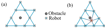
Fig. 3. Configurations with (a) 14 edges, (b) 18 edges. The red robot in (b) tends to collide with obstacles due to attractions from extra neighbors.
