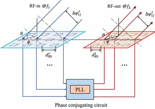
Fig. 3. Schematic diagram of the principle of RB-ISAC echo signal original path return.
