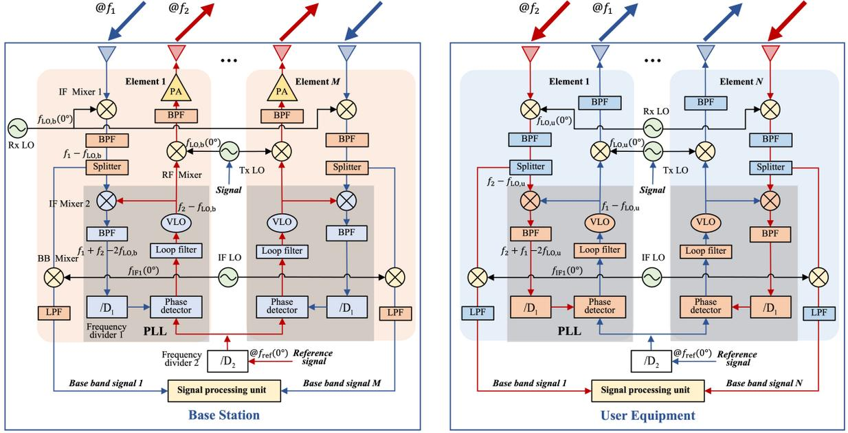
Fig. 2. Diagram of uplink and downlink frequency separation structure and conjugate circuit structure in resonant beam-based integrated localization and communication system.
