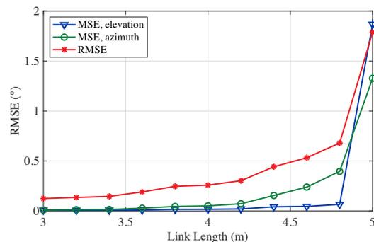
Fig. 12. The RMSE of RB-SLAC system in different link length.
