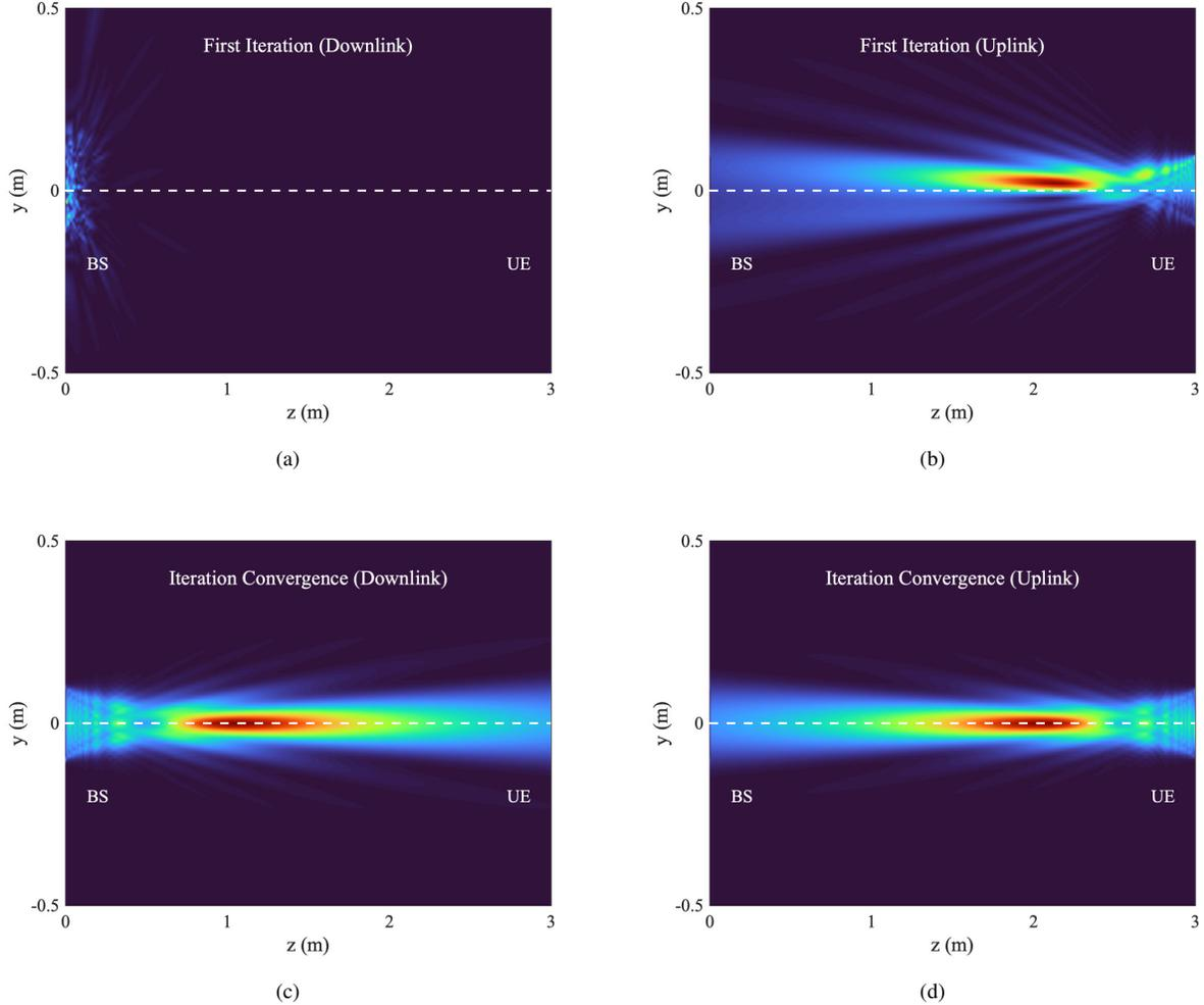
Fig. 5. Normalized distribution of spatial signal strength in  $xoz$ -plane. (a) Distribution of signal strength for the first transmission of the downlink; (b) The strength distribution of the first transmission signal on the uplink; (c) After the system reaches steady state, the distribution of downlink signal strength; (d) After the system reaches steady state, the distribution of uplink signal strength.
