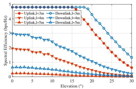
Fig. 9. Spectrum efficiency analysis with different elevation.
