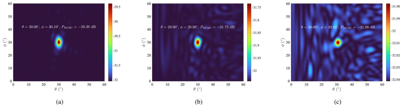
Fig. 10. The DOA estimation results of RB-ISAC system at different link lengths have true value of  $\theta = \phi = 30^\circ$ . (a)  $l=3\text{m}$ ; (b)  $l=4\text{m}$ ; (c)  $l=5\text{m}$ .
