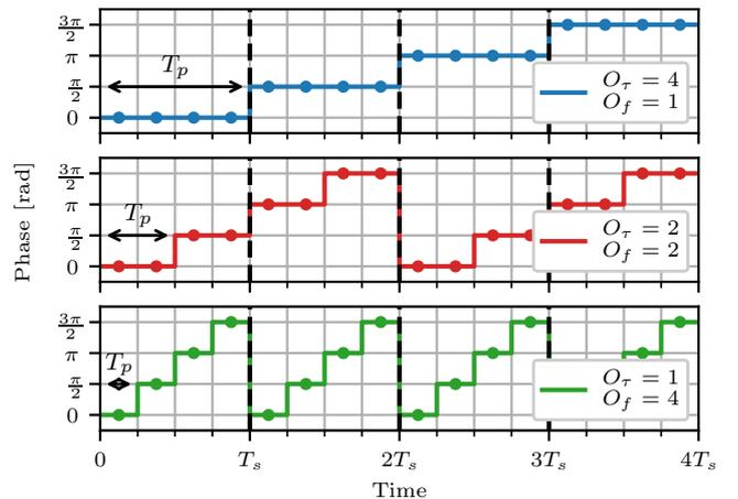
Fig. 2. Modulating signal in the time domain with upsampling factor  $O = 4$  and number of phase shift values  $N = 4$  for selected pulse duration and modulation frequency scaling factors, where  $T_s = 1/f_s$  is the sample period.
