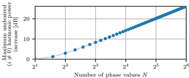
Fig. 7. Worst-case undesired harmonic ( $i \neq 0$ ) power increase while tapering as compared to the case without tapering as a function of the number of phase shift values  $N$ .
