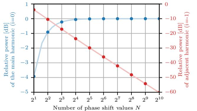
Fig. 4. Power of the main harmonic ( $i = 0$ ) and strongest undesired harmonic ( $i = -1$ ) as a function of the number of phase shift values.
