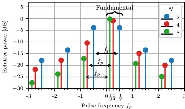
Fig. 3. Power per harmonic component for modulating sequences with a selected number of phase shift values  $N = 2, 4, 8$ .
