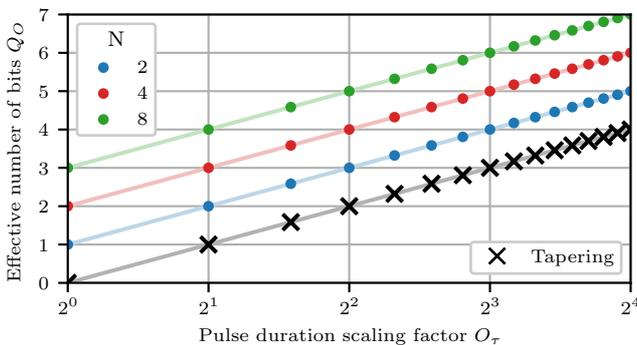
Fig. 5. Effective number of bits as a function of pulse duration scaling factor  $O_\tau$  for a selected number of phase shifts  $N$ .
