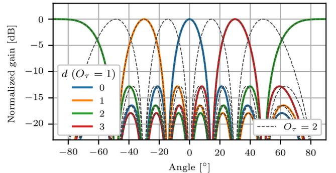
Fig. 6. Beam pattern of the main harmonic component ( $i = 0$ ) per delay value for  $M = 8$  antennas,  $N = 4$  and two values of pulse duration scaling factor  $O_\tau = 1, 2$ .
