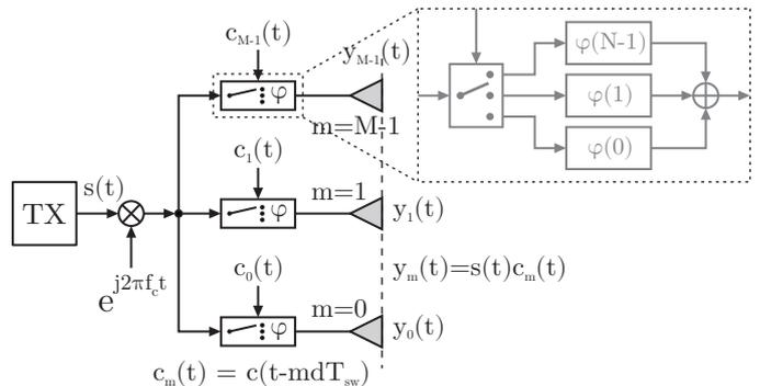
Fig. 1. Architecture of the time-modulated array. Each antenna is preceded by an  $N$ -state switch which acts as a discrete phase shifter. The delay of the modulating sequence, which creates the modulating signal, is adjusted per antenna facilitating digital beamforming.
