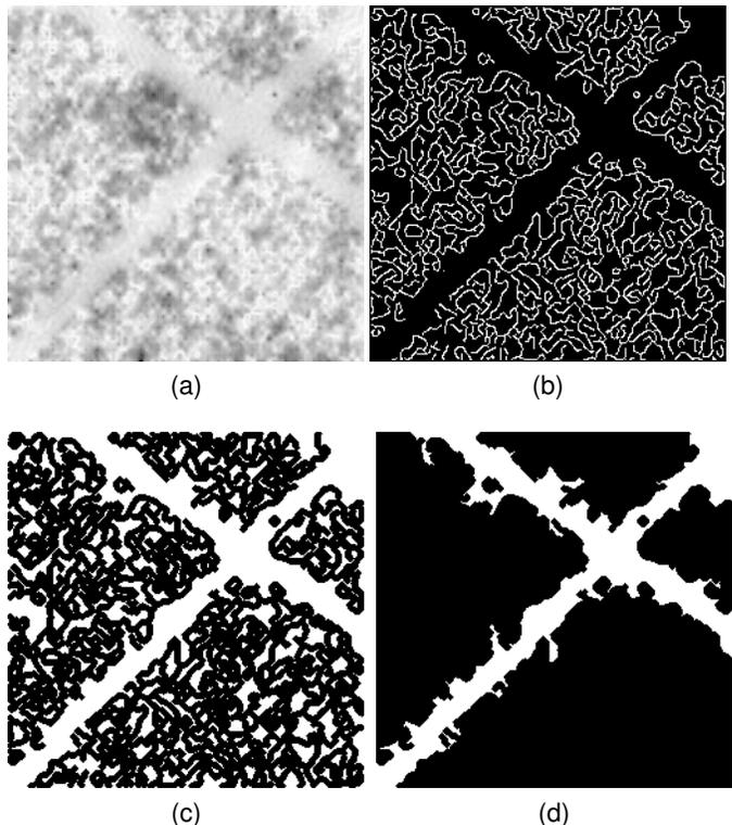
Fig. 3. Image processing steps; (a) Gray scale image (b) Edge filter (c) Dilation (d) Connected components.
