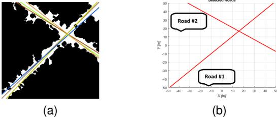
Fig. 4. Parameter extraction: (a) Image with detected lines; (b) Road parameters:  $(\rho_1, \alpha_1) = (0, 45^\circ)$  and  $(\rho_2, \alpha_2) = (25, -35^\circ)$ .
