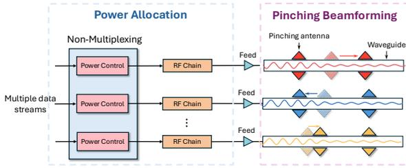
Fig. 2: Non-Multiplexing transmission architectures for PASS
