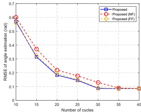
Fig. 5. Angle estimation performance versus number of cycles for FF users.
