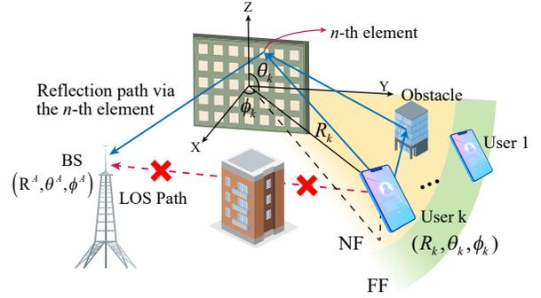
Fig. 1. RIS-enabled multi-user localization system.
