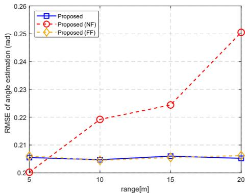
Fig. 6. Angle estimation performance versus localization ranges for FF users.
