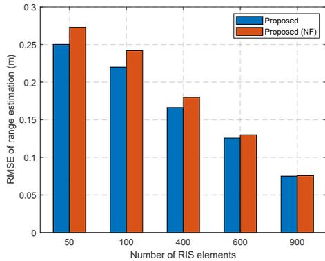
Fig. 10. Range estimation performance of the NF users versus RIS size.<sup>1</sup>
