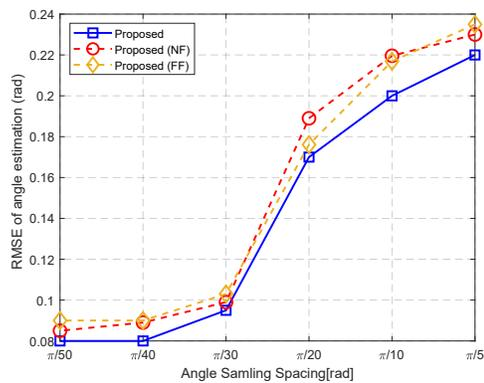
Fig. 8. Average angle estimation performance of the NF and FF users for different angle sampling spacing.
