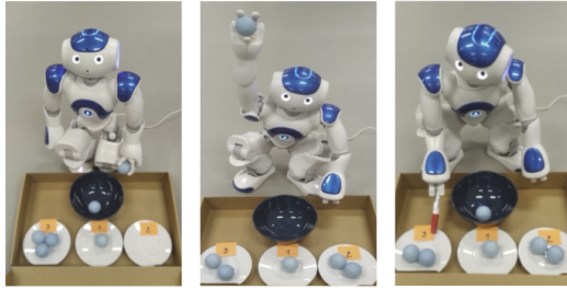
Figure 7: Examples of converting a planned action into a real robot action according to the selected teaching strategy: moving the object to a target location, passing the object to the student and pointing to the object.
