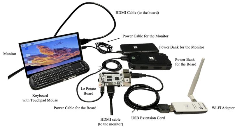
Figure 4. Hardware setup
