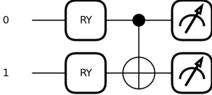
Figure 2: Quantum Kernel Circuit. The circuit demonstrates the combination of parameterized rotations ( $RY$ ) and the Controlled-NOT (CNOT) gate used to compute quantum token similarities.
