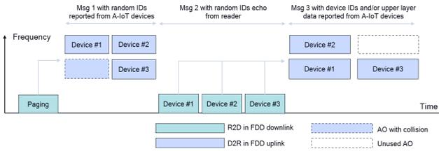
**Fig. 1.** A-IoT CBRA procedure and time-frequency arrangement
