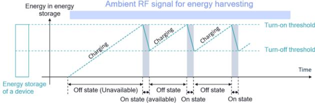
Fig. 2.  $e_{es}$  with A-IoT device on/off states
