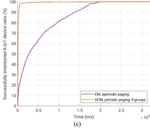
**Fig. 5.** (a) CDF of  $p_{in}$  (dBm) in the layout; (b) ratio of A-IoT devices that have successfully been inventoried in time (device 1); (c) ratio of A-IoT devices that have successfully been inventoried in time (device 2)
