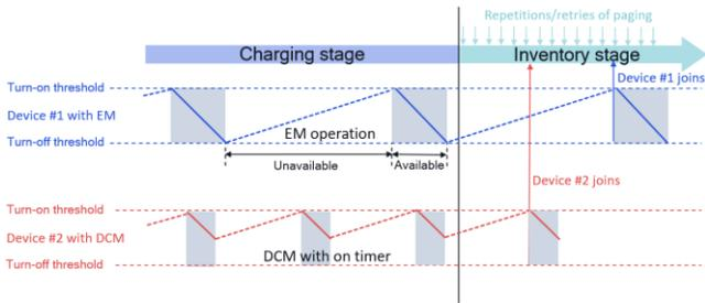
Fig. 3. Comparison of EM mechanism and DCM mechanism.
