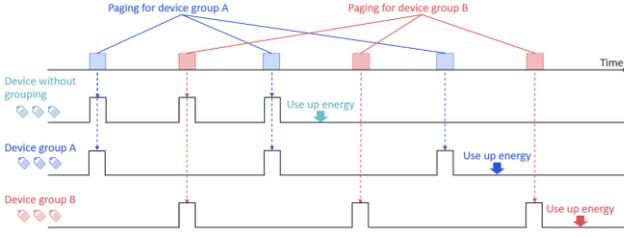
**Fig. 4.** Illustration of device grouping
