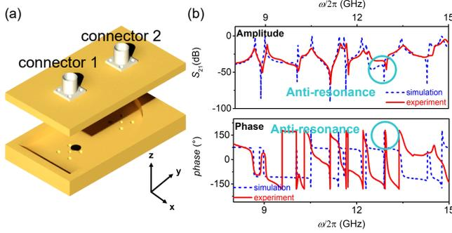
FIG. 4. (a) Schematic diagram of the experimental device (quadrant-stadium cavity). The position of the YIG wafer is (20 mm, 15 mm, 0 mm). The spectrum is measured using VNA through connector 1 and connector 2. (b) The amplitude and phase of of the rectangular cavity without applied magnetic field from 8 GHz to 15 GHz. The red solid line and the blue dashed line stands for the experiment data and the simulation data, respectively.
