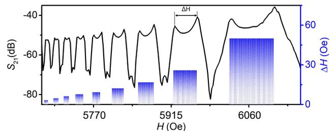
FIG. 6. The black solid line represents the change of the transmission parameter with the applied magnetic field at the anti-resonance frequency of 13.05 GHz. The blue histogram stands for the variation trend of  $\Delta H$ .
