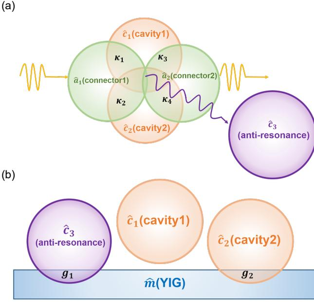
FIG. 1. (a) Schematic diagram of the anti-resonance generated by the joint action of connectors and cavity modes. (b) Schematic diagram of magnon-photon couplings in this work.  $\hat{c}_1$  and  $\hat{c}_2$  are the cavity modes.  $\hat{c}_3$  is anti-resonance mode.  $\hat{a}_1$  and  $\hat{a}_2$  are the connector modes.  $\hat{m}$  is the magnon mode.
