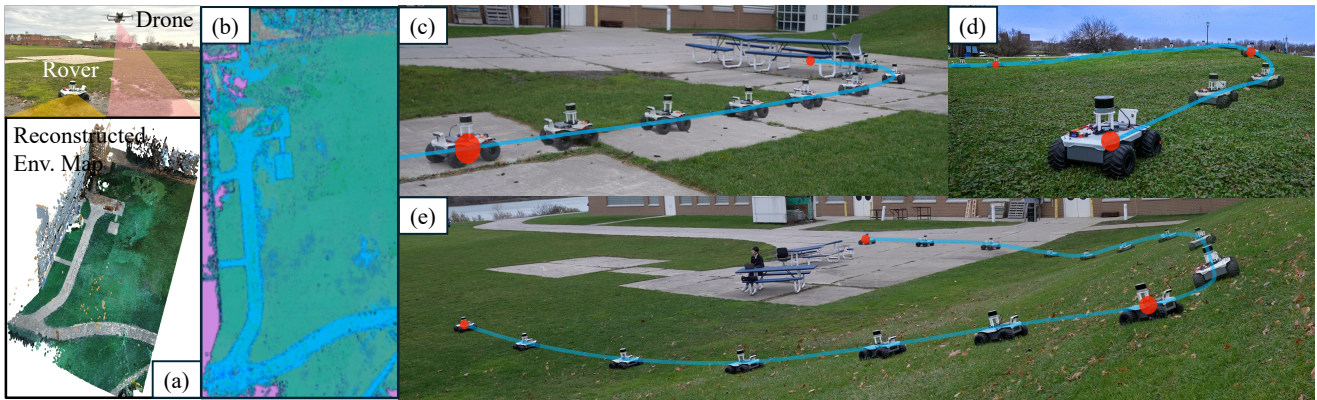
Figure 20. Real-world deployment of our AnyNav system. (a) The environment map is collaboratively reconstructed by a rover and a drone. (b) The Stribeck coefficient is estimated using the neuro-symbolic module. (c-e) Multiple navigation tasks are executed using the AnyNav planner. The red points are selected target locations and the blue lines are planned trajectories.
