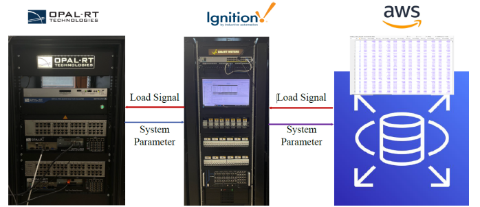
Fig. 3: Our Hardware in the loop infrastructure: Left: Hardware simulator, middle: SCADA interface, right: Real-Time database
