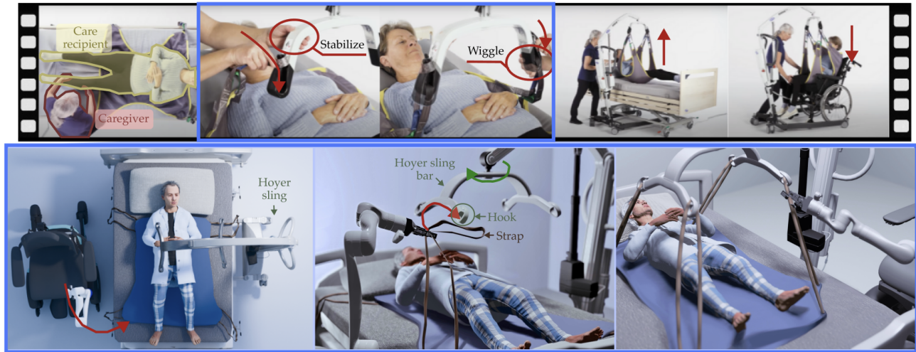
Fig. 1: Bed-to-wheelchair Transferring : Human caregivers use assistive devices to perform transferring. For example, the caregiver in the figure (upper row) uses a Hoyer sling to move the care recipient from the hospital bed to the wheelchair. Inspired by this, we use an instrumented Hoyer sling along with a caregiving robot to perform the transferring task (lower row), where the robot performs fine manipulation, and the assistive devices take the heavy loads.
