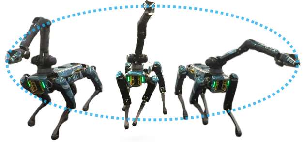
Fig. 1: Boston Dynamics Spot with an attached arm tracking an ellipsoidal reference trajectory with its end-effector in our experiments.
