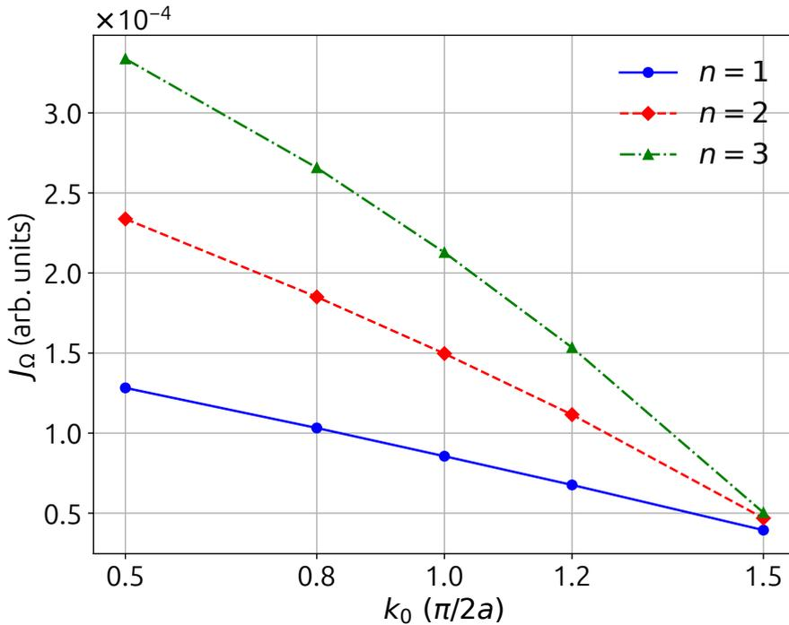
Figure 5.24: Variation in the anomalous current's maximum amplitude along  $y$  axis, which is solely due to the Berry curvature,  $\mathbf{J}_\Omega$ , as a function of the separation between two Weyl nodes,  $k_0$ , for different topological charges  $n$ . The laser parameters are identical as in Fig. 5.22 except the intensity  $10^8$  W/cm<sup>2</sup>.
