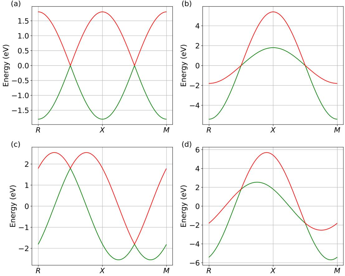
Figure 5.12: Energy bands corresponding to time-reversal symmetry broken Weyl semimetal along high-symmetry directions  $R(0, 0, \pi/a) \rightarrow \Gamma(0, 0, 0) \rightarrow M(0, 0, -\pi/a)$  for (a)  $t_c = t_g = 0$ , (b)  $t_c = 2$  and  $t_g = 0$ , (c)  $t_c = 0$  and  $t_g = 1$  and (d)  $t_c = 2$  and  $t_g = 1$ . The Fermi level is set at zero energy in all cases.
