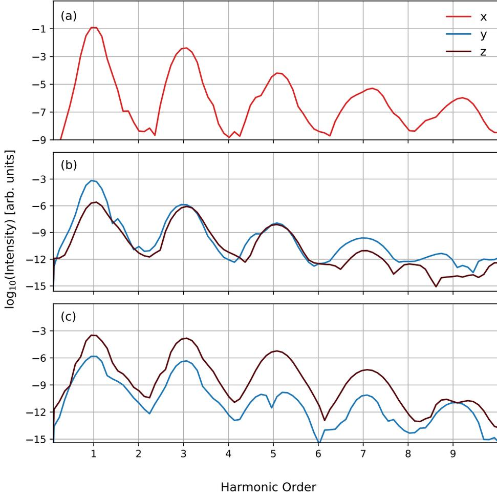
Figure 5.2: High-harmonic spectra corresponding to a linearly polarized pulse. The pulse is polarized along (a)  $x$ , (b)  $y$ , and (c)  $z$  directions. Driving pulse is  $\simeq 100$  fs long with intensity  $1 \times 10^{11}$  W/cm<sup>2</sup>, and wavelength  $3.2 \mu\text{m}$ . Decoherence time of 1.5 fs is added phenomenologically.
