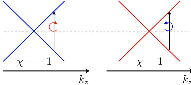
Figure 2.8: Selective excitation of the Weyl cones by circularly polarized light. The left helicity of light excites the Weyl cone with chirality  $\chi = -1$  in the  $+k_z$  direction, and the same side of the Weyl cone with chirality  $\chi = 1$  can be excited by the right helicity of light.
