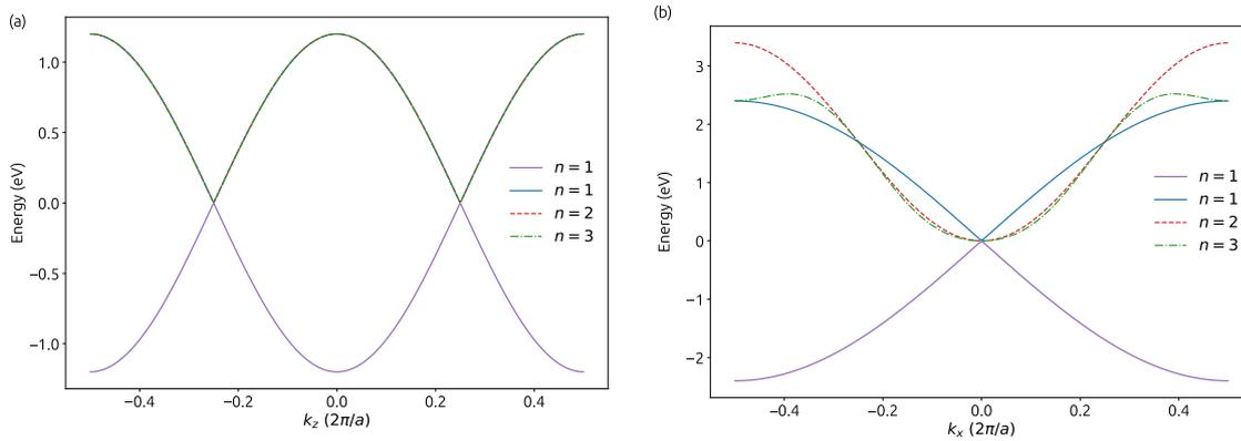
Figure 5.18: Energy bands corresponding to m-WSMs with different topological charges along (a) the  $k_z$  direction, and (b) the  $k_x$  direction around a Weyl node. The band structures along the  $k_y$  and  $k_x$  directions are identical. The band structure is obtained by diagonalizing  $\mathcal{H}^{(n)}$  with the hopping parameter  $t = 1.2 \text{ eV}$  and the lattice parameter  $a = 6.28 \text{ \AA}$ . The purple line corresponds to the valence band in all cases.
