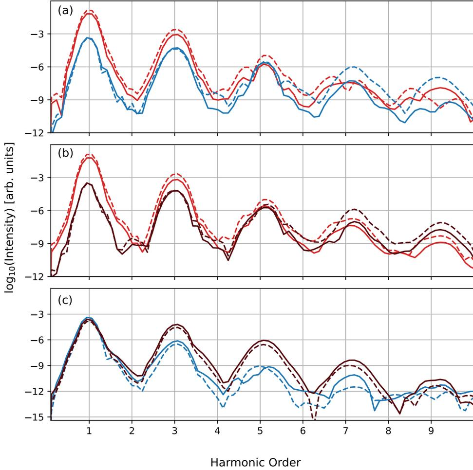
Figure 5.9: Comparison of the parallel harmonic yield for two different values of  $k_0$ . The laser is circularly polarized in (a)  $xy$ , (b)  $xz$ , and (c)  $yz$ - planes. Red, blue and brown correspond to  $x$ ,  $y$  and  $z$  polarization, respectively. Solid (dotted) line represents the value of  $k_0 = \pm 0.2(\pm 0.3)$ . The value of  $k_0$  is varied from  $\pm 0.2$  to  $\pm 0.3$  rad/au.
