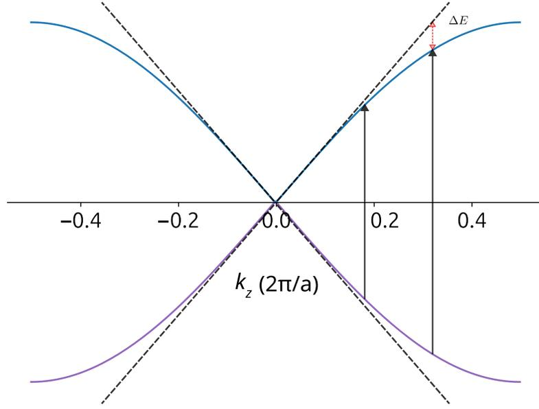
Figure A.1: Deviation of the energy band dispersion beyond the linear behaviour around a Weyl node.
