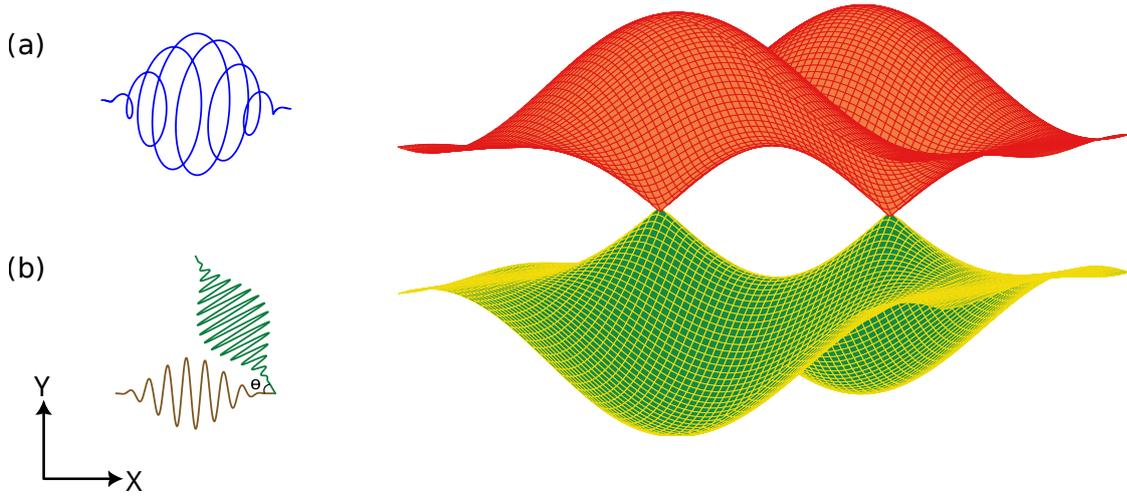
Figure 4.1: Schematic setup for ultrafast photocurrent generation in a solid, which is represented by an inversion-symmetric Weyl semimetal. (a) A circularly-polarized laser with frequency  $\omega$  is interacting to a solid. (b) Alternatively, two linearly-polarized pulses with frequencies  $\omega$  and  $2\omega$  with polarization directions at an angle  $\theta$  are interacting with the solid.
