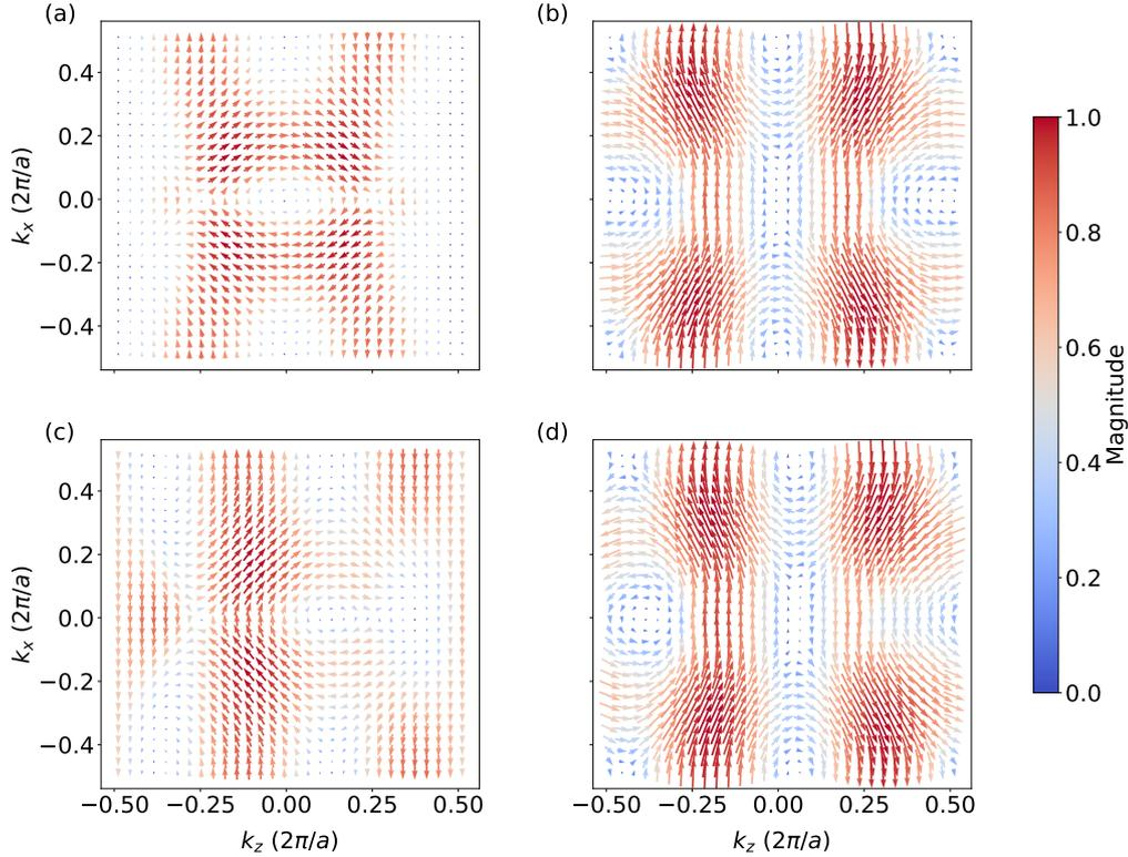
Figure 5.15: Momentum matrix element  $\mathbf{p}_{cc}^{\mathbf{k}} = \langle c, \mathbf{k} | \nabla_{\mathbf{k}} \mathcal{H}_{\text{Weyl}}(\mathbf{k}) | c, \mathbf{k} \rangle$  with  $|c, \mathbf{k}\rangle$  as the eigenstate of the conduction band of time-reversal symmetry broken Weyl semimetal for (a)  $t_c = t_g = 0$ , (b)  $t_c = 2$  and  $t_g = 0$ , (c)  $t_c = 0$  and  $t_g = 1$  and (d)  $t_c = 2$  and  $t_g = 1$ .
