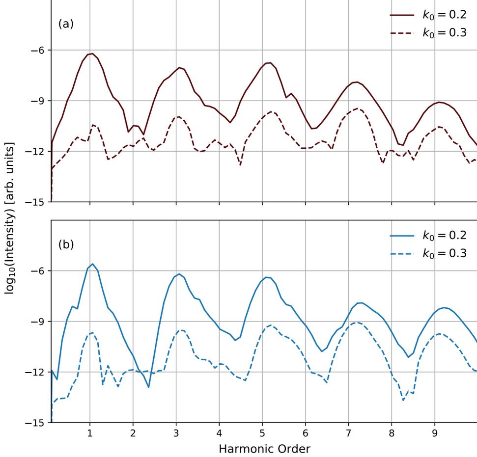
Figure 5.5: Comparison of the anomalous high-harmonic yield for different values of  $k_0$ , which is proportional to the distance between the two Weyl points. Odd anomalous harmonics along (a)  $z$  direction when polarization of the pulse is in  $xy$ - plane, and (b)  $y$  direction when polarization of the pulse is in  $xz$ - plane.
