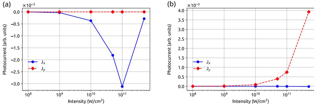
Figure 4.18: Scaling of the photocurrent with the intensity of the  $\omega$  and  $2\omega$  pulses in (a) collinear and (b) orthogonal configurations with  $\mathcal{R} = 1$  and  $0.5$ , respectively. The laser parameters are the same as in Fig. 4.12 for an inversion-symmetric Weyl semimetal.
