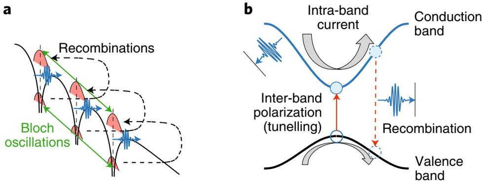
Figure 1.3: Mechanism of high-harmonic generation in solids: (a) A real-space view showing tunneling, Bloch oscillation, and recombination, (b) reciprocal-space picture showing the three steps: 1. tunneling (interband transition), 2. intra-band motion, and 3. recombination. This figure is adapted from (Ghimire and Reis, 2019).
