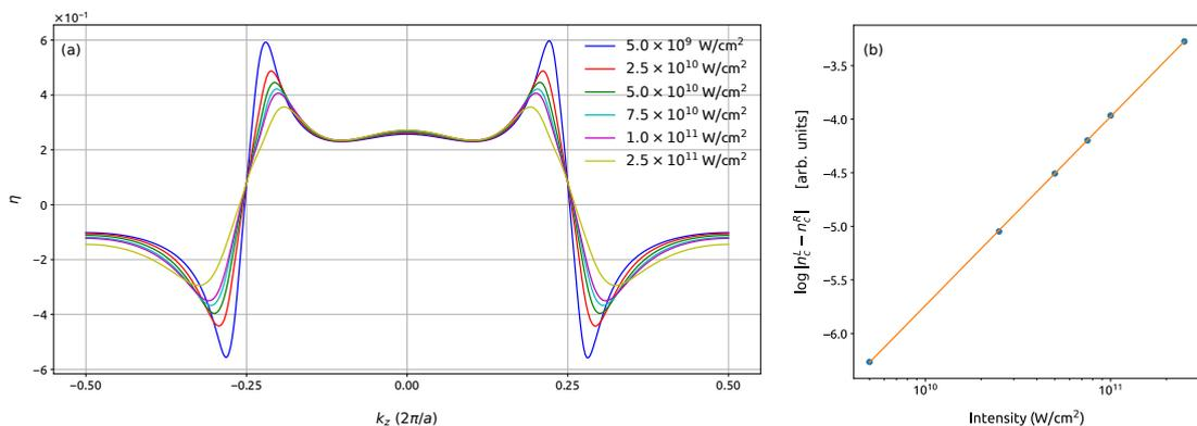
Figure 3.5: (a) Variations of  $\eta$  for different intensities of the circularly polarized light. (b) Logarithm of the difference in the population around a given Weyl node excited by the left- or right-handed circularly polarized light as a function of the laser's intensity. The slope of the fitted line is 0.8, i.e., is below unity expected for linear processes. The driving light wavelength is 3.2  $\mu\text{m}$ . The simulations use the full Hamiltonian given in Eq. (3.1.1).
