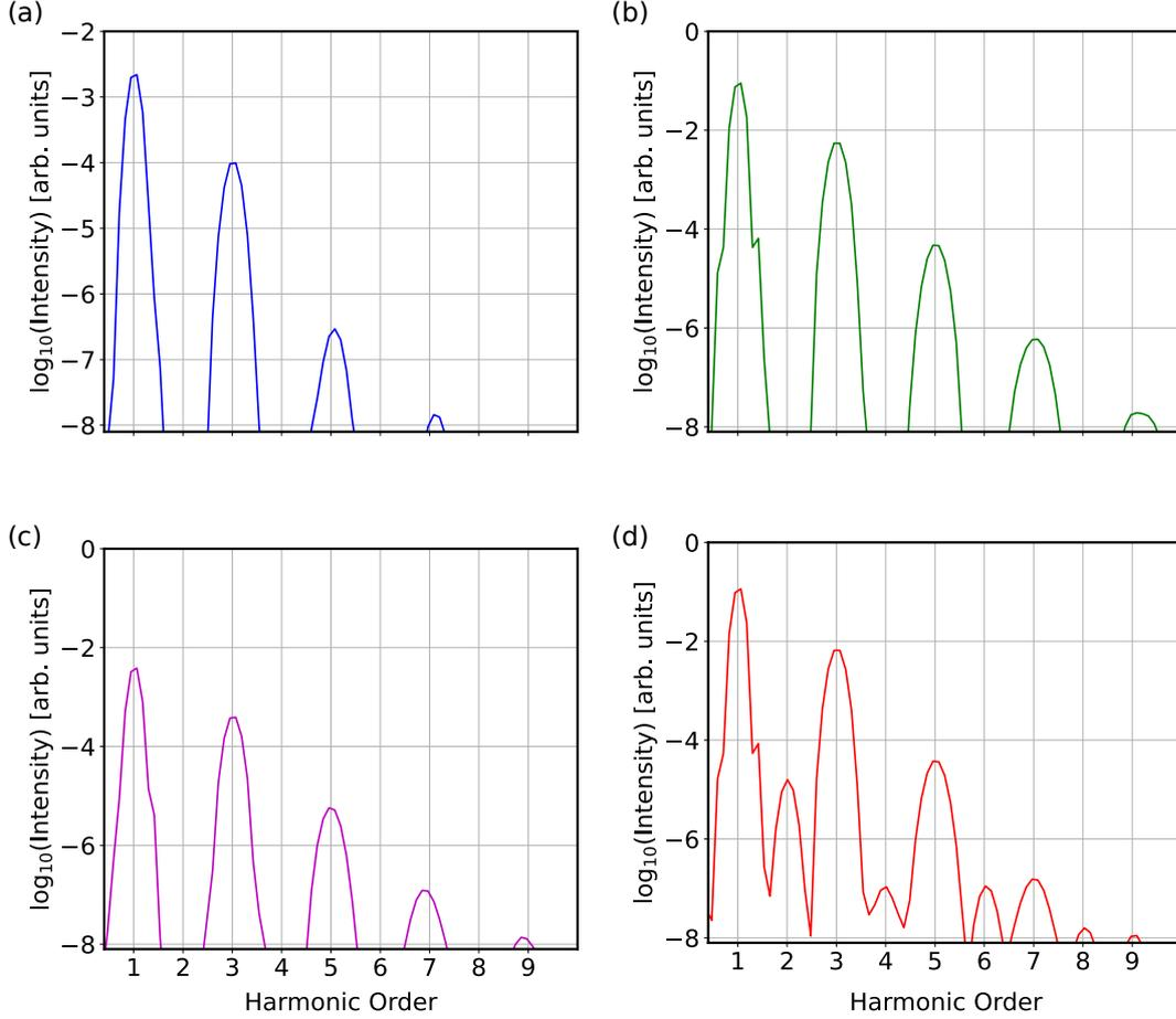
Figure 5.13: High-harmonic spectra of time-reversal symmetry broken Weyl semimetal for (a)  $t_c = t_g = 0$ , (b)  $t_c = 2$  and  $t_g = 0$ , (c)  $t_c = 0$  and  $t_g = 1$  and (d)  $t_c = 2$  and  $t_g = 1$ . The peak intensity of the laser is  $10^{11}$  W/cm<sup>2</sup> with 3.2  $\mu\text{m}$  wavelength and about 80 fs long.
