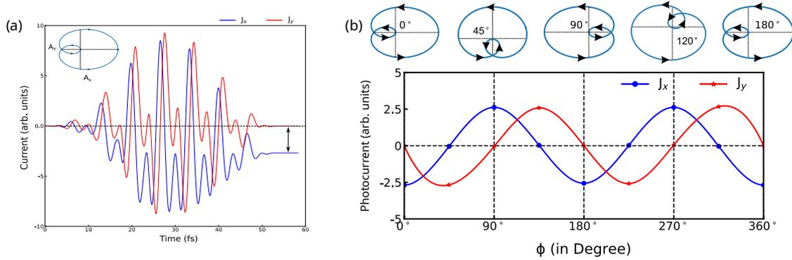
Figure 1.2: Laser-driven photocurrent in pristine graphene: (a)  $\omega - 2\omega$  co-rotating circularly polarized pulses have asymmetric waveform (shown in inset) and hence lead to photocurrent along  $x$  direction. (b) By tuning the relative phase between  $\omega$  and  $2\omega$  pulses, the waveform is changed to tailor the directions and magnitude of the photocurrent in graphene. This figure is adapted from (Rana and Dixit, 2024).
