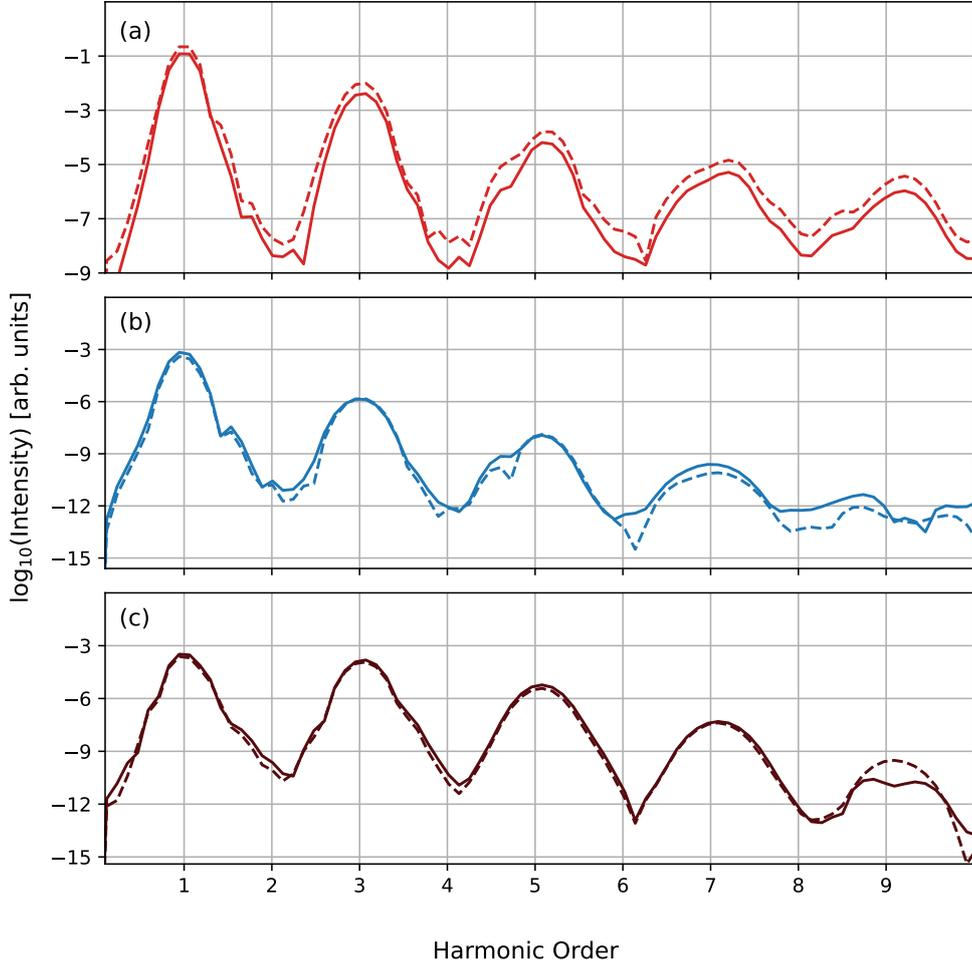
Figure 5.8: Comparison of the parallel harmonic yield for two different values of  $k_0$ . The laser is polarized along (a)  $x$ , (b)  $y$ , and (c)  $z$  directions. Red, blue and brown correspond to  $x$ ,  $y$  and  $z$  polarization, respectively. Solid (dotted) line represents the value of  $k_0 = \pm 0.2(\pm 0.3)$ . The value of  $k_0$  is varied from  $\pm 0.2$  to  $\pm 0.3$  rad/au.
