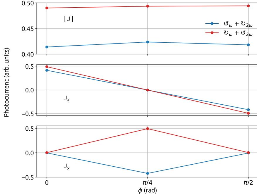
Figure 4.11: Variation in the photocurrent and its components in an inversion-symmetric Weyl semimetal, described by Eq. (4.1.1) with respect to the sub-cycle phase between  $\omega - 2\omega$  fields. Eight-cycle laser pulse with its fundamental wavelength of  $3.2 \mu\text{m}$  and intensity of  $0.5 \times 10^{10} \text{ W/cm}^2$  is used.
