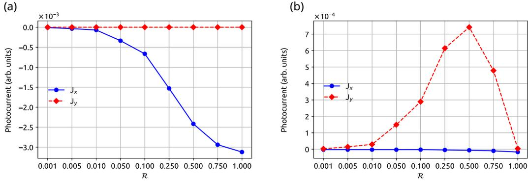
Figure 4.13: Variation in photocurrent with the amplitude ratio ( $\mathcal{R}$ ) of the  $2\omega$  pulse with respect to the  $\omega$  pulse for an inversion-symmetric Weyl semimetal in the (a) collinear and (b) orthogonal configurations. Laser parameters are the same as in Fig. 4.12 with intensity of the  $\omega$  pulse as  $10^{11}$  W/cm<sup>2</sup>.
