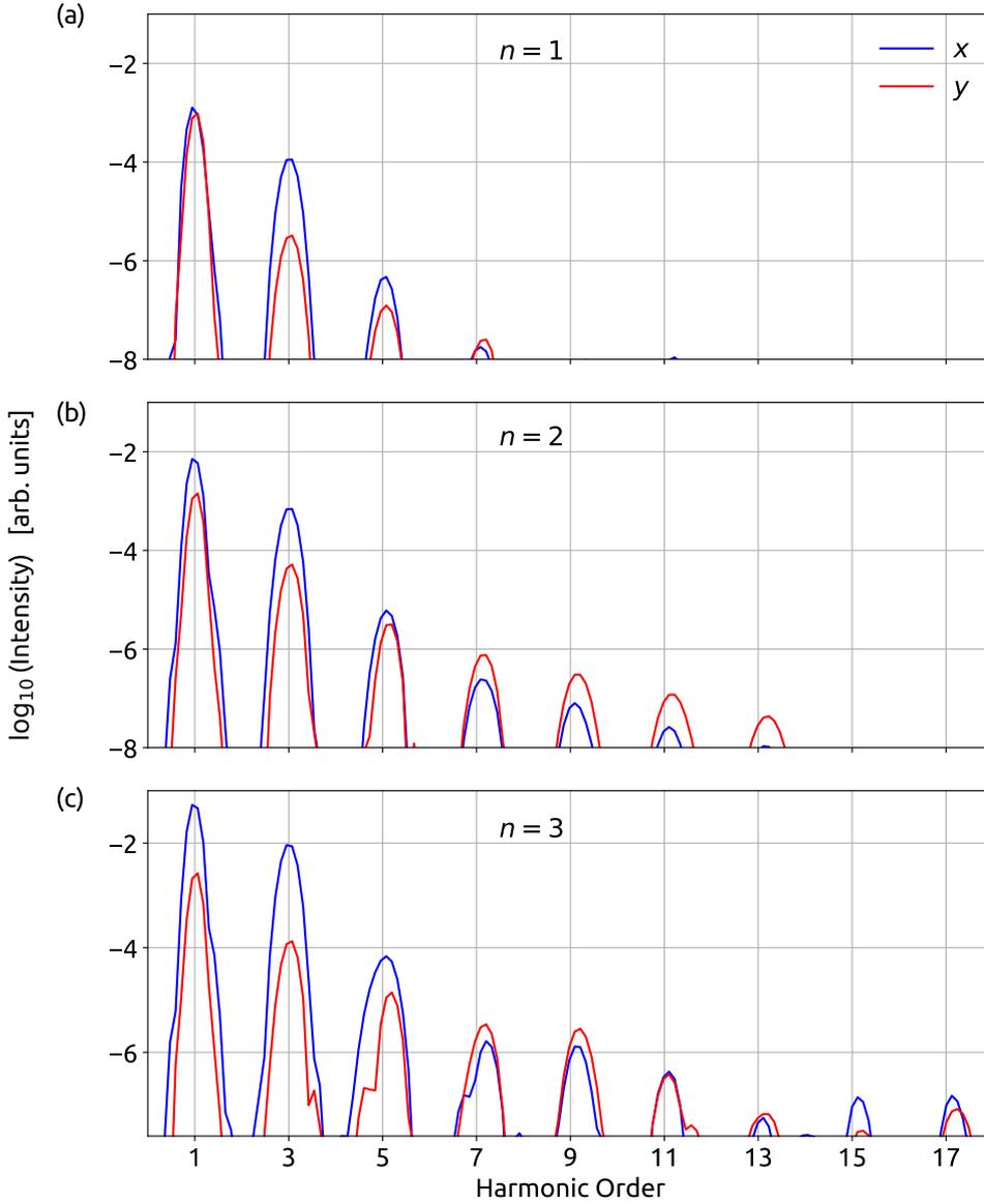
Figure 5.25: High-harmonic spectrum corresponding to m-WSMs with topological charge (a)  $n = 1$ , (b)  $n = 2$ , and (c)  $n = 3$ . The driving laser is 100 fs long with wavelength of  $3.2 \mu\text{m}$  and intensity of  $10^{11} \text{ W/cm}^2$ . The laser pulse is linearly polarized along  $x$  direction. A phenomenologically decoherence time of 1.5 fs is added.
