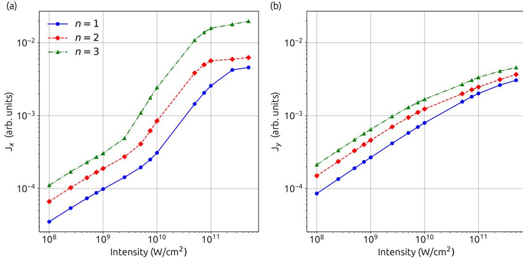
Figure 5.20: Variations of the maximum amplitude for (a) the normal current along  $x$  and (b) the anomalous current along  $y$  as a function of the laser's intensity for m-WSMs with topological charges  $n = 1, 2$ , and 3. The other parameters are the same as those in Fig. 5.19.
