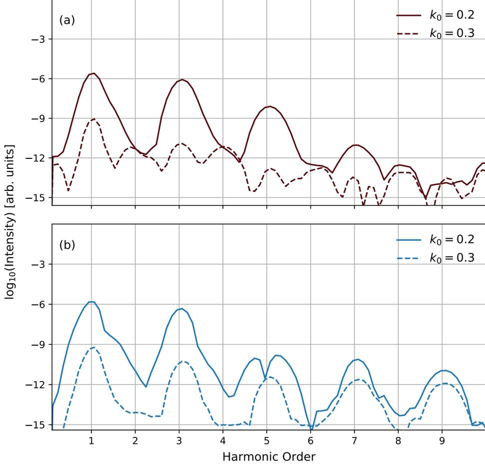
Figure 5.7: Comparison of the anomalous harmonic yield for two different values of  $k_0$ . Odd anomalous harmonics along (a)  $z$  direction when laser is linearly polarized along  $y$  direction, and (b) along  $y$  direction when laser is linearly polarized along  $z$  direction. The value of  $k_0$  is varied from  $\pm 0.2$  to  $\pm 0.3$  rad/au.
