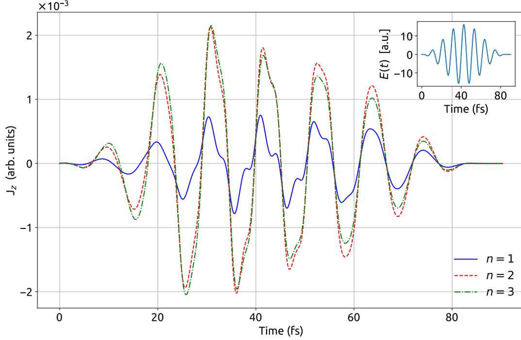
Figure 5.17: Total current along the  $z$  direction in m-WSMs for different topological charges  $n$ . The linearly polarized laser pulse along the  $z$  direction is employed to generate the current and is shown in the inset. The laser is approximately 100 fs long with a wavelength of  $3.2 \mu\text{m}$  and an intensity of  $10^{11} \text{ W/cm}^2$ . The value of the phenomenologically decoherence time is 1.5 fs.
