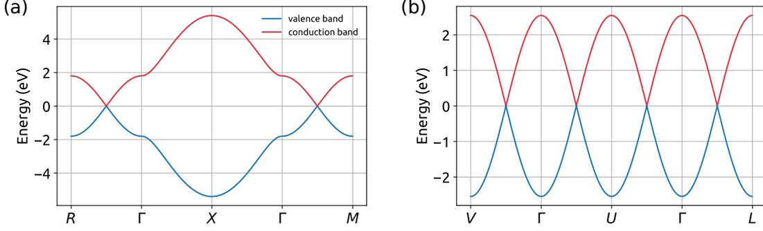
Figure 4.2: (a) Energy dispersion of an inversion-symmetric Weyl semimetal, described by Eq. (4.1.1) along high-symmetry path  $R(0, 0, \pi/a) \rightarrow \Gamma(0, 0, 0) \rightarrow X(\pi/a, 0, 0) \rightarrow M(0, 0, -0.5)$ . (b) Energy dispersion of an inversion-broken Weyl semimetal, described by Eq. (4.1.2) along high-symmetry path  $V(\pi/a, -\pi/a, 0) \rightarrow \Gamma(0, 0, 0) \rightarrow U(\pi/a, \pi/a, 0) \rightarrow L(-\pi/a, -\pi/a, 0)$ .
