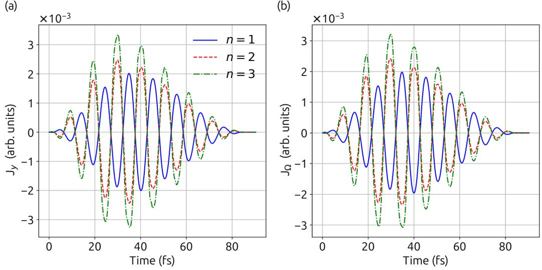
Figure 5.22: (a) Total current along  $y$  direction, (b) current solely due to the Berry curvature along  $y$  direction for different topological charges  $n$ . The laser is approximately 100 fs long with wavelength of  $3.2 \mu\text{m}$  and intensity of  $10^{11} \text{ W/cm}^2$ . The laser pulse is linearly polarized along  $x$  axis.
