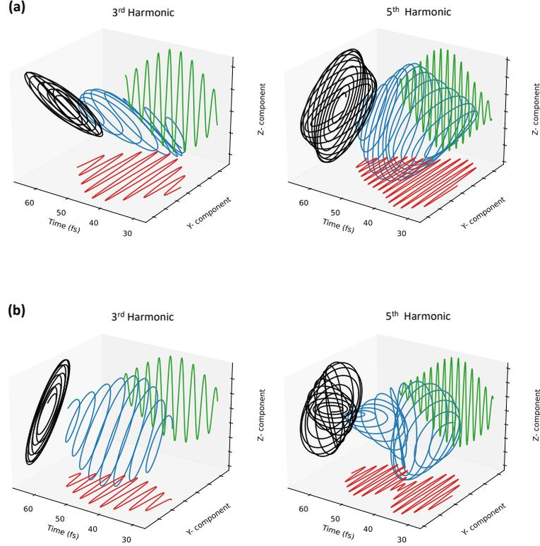
Figure 5.10: The total time-dependent electric field (in blue) corresponding to third and fifth harmonics in time-reversal broken Weyl semimetal. The  $y$ -component (in red),  $z$ -component (in green), and Lissajous figure (in black). The harmonics in Weyl semimetal are generated using linearly polarized pulse along (a)  $y$ -axis and (b)  $z$ -axis as shown in Figs. 5.2(b) and 5.2(c), respectively.
