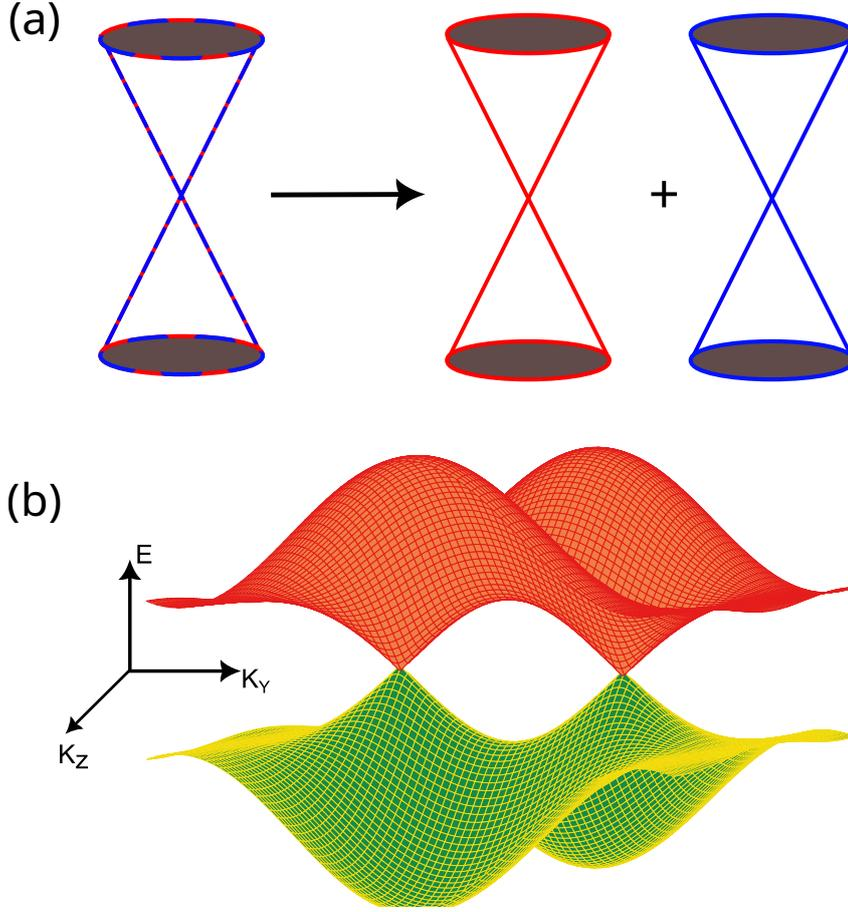
Figure 2.6: (a) Dirac points have copies of two chiralities superimposed, which can be separated into two Weyl points by breaking inversion or time-reversal symmetry. (b) Band structure of a generic Weyl semimetal with “at least” two band-touching, or Weyl nodes.
