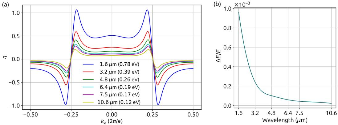
Figure 3.4: (a) Normalized population asymmetry ( $\eta$ ) as a function of the wavelength of the circularly polarized pulse with intensity  $5 \times 10^9 \text{ W/cm}^2$ . (b) Nonlinear correction ( $\Delta E$ ) to the energy ( $E$ ) obtained from the linear dispersion. The simulations use the full Hamiltonian given in Eq. (3.1.1).
