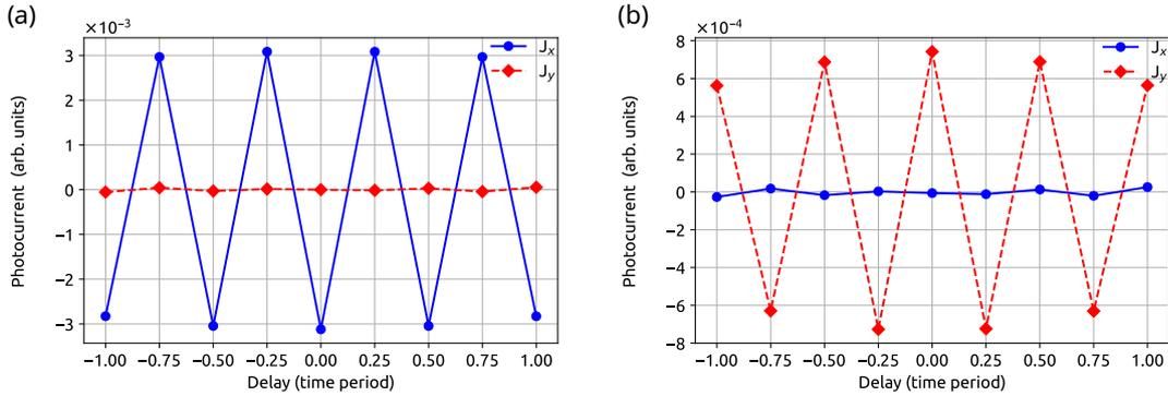
Figure 4.17: Effect of the time-delay between of  $\omega$  and  $2\omega$  pulses on the photocurrent in an inversion-symmetric Weyl semimetal. The  $\omega$  and  $2\omega$  pulses are in (a) collinear and (b) orthogonal configurations with  $\mathcal{R} = 1$  and  $0.5$ , respectively. The laser parameters are the same as in Fig. 4.12.
