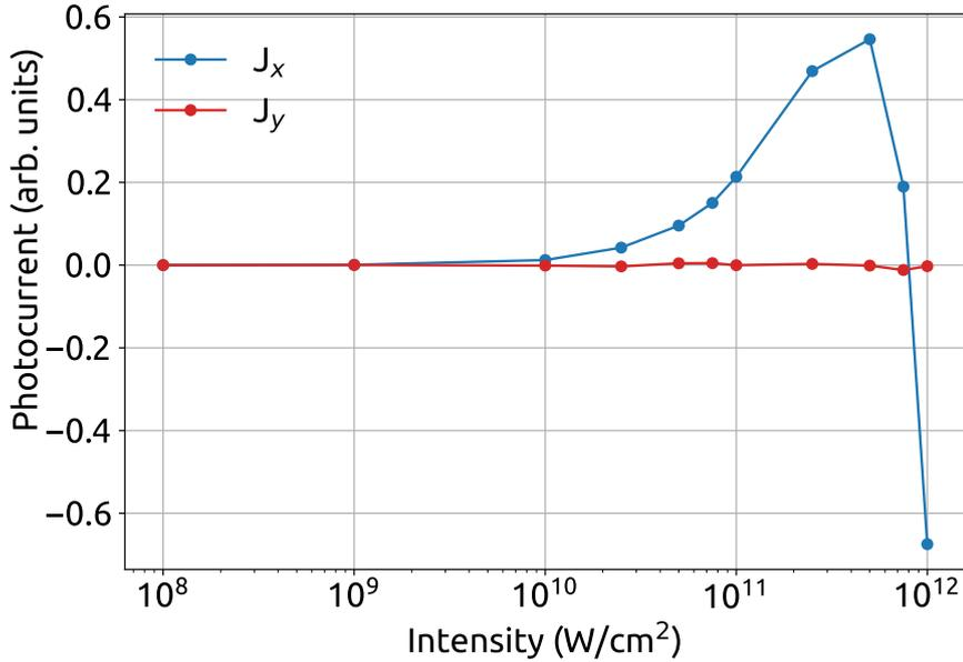
Figure 4.8: Scaling of the photocurrent in an inversion-symmetric Weyl semimetal with the laser's intensity of the right-handed circularly polarized light with  $\phi = 0$ . The other laser parameters are same as Fig. 4.3.
