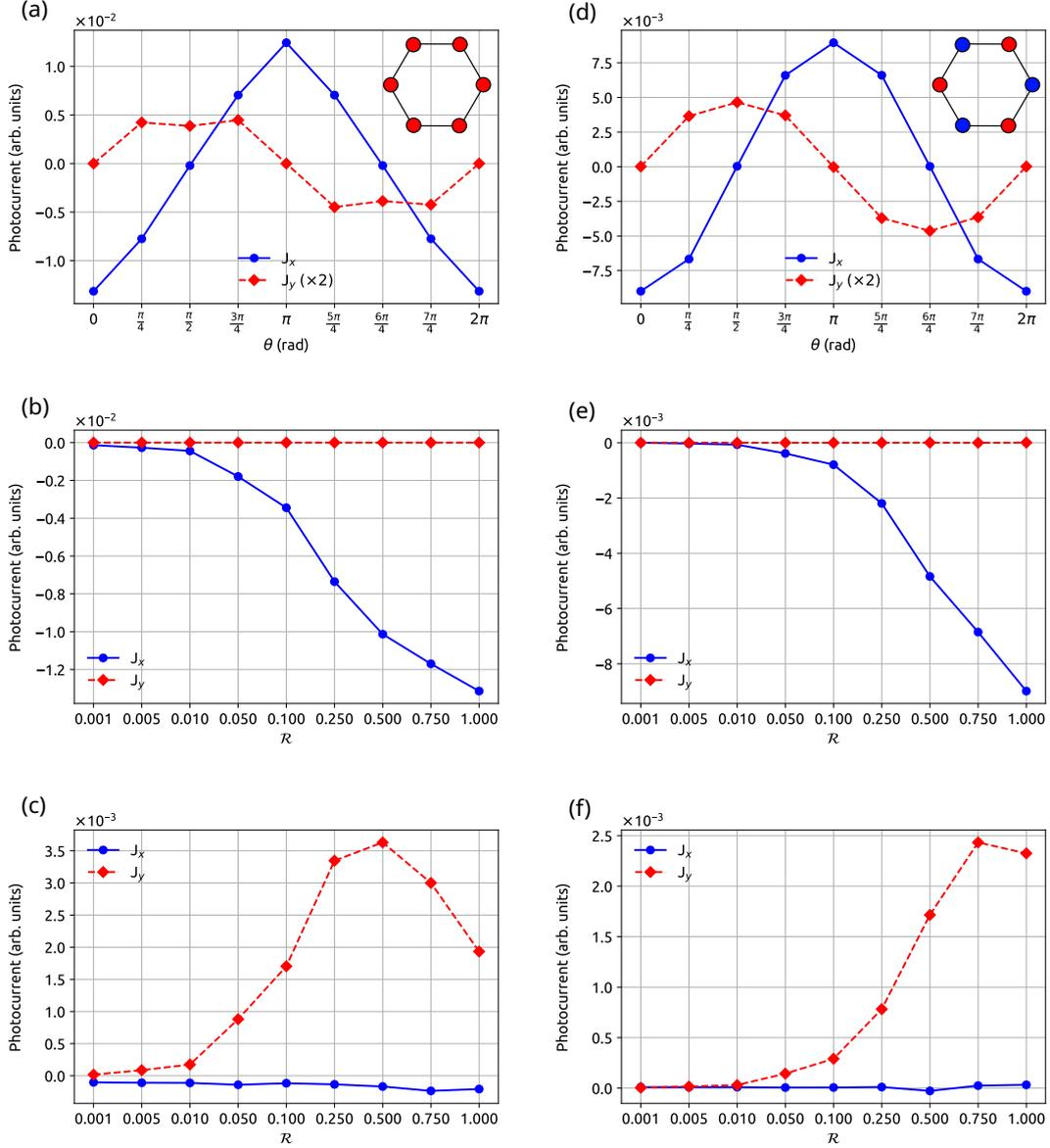
Figure 4.16: (a) Sensitivity of the photocurrent in an inversion-symmetric graphene with respect to (a)  $\theta$ , the amplitude ratio ( $\mathcal{R}$ ) in (b) collinear and (c) orthogonal configurations of the  $\omega - 2\omega$  setup. Panels (d), (e), and (f) are the same as (a), (b), and (c) for MoS<sub>2</sub>, respectively. Laser parameters are the same as in Fig. 4.12 with intensity of the  $\omega$  pulse as  $10^{11}$  W/cm<sup>2</sup>.
