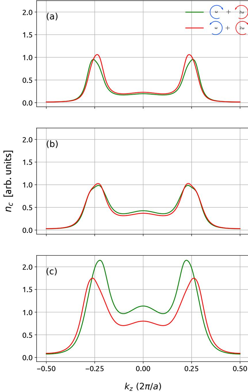
Figure 3.6: Residual population for different ratio ( $\mathcal{R}$ ) of the two-color  $\omega - 2\omega$  laser pulses: (a)  $\mathcal{R} = 0.2$ , (b)  $\mathcal{R} = 0.5$ , and (c)  $\mathcal{R} = 1.0$ . Intensity and wavelength of the  $\omega$  pulse are  $5 \times 10^{10}$  W/cm<sup>2</sup> and 3.2  $\mu\text{m}$ , respectively.
