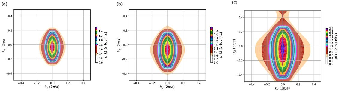
Figure 4.14: Residual electronic population in the conduction band after the end of the laser pulse for (a)  $\mathcal{R} = 0.1$ , (b)  $\mathcal{R} = 0.25$  and (c)  $\mathcal{R} = 1.0$ . The population along  $k_z$  direction is integrated as the  $\omega - 2\omega$  field setup lies on the  $k_x - k_y$  plane. Note that the scale of the color bar is different in all cases. Rest of the parameters are same as Fig. 4.12.
