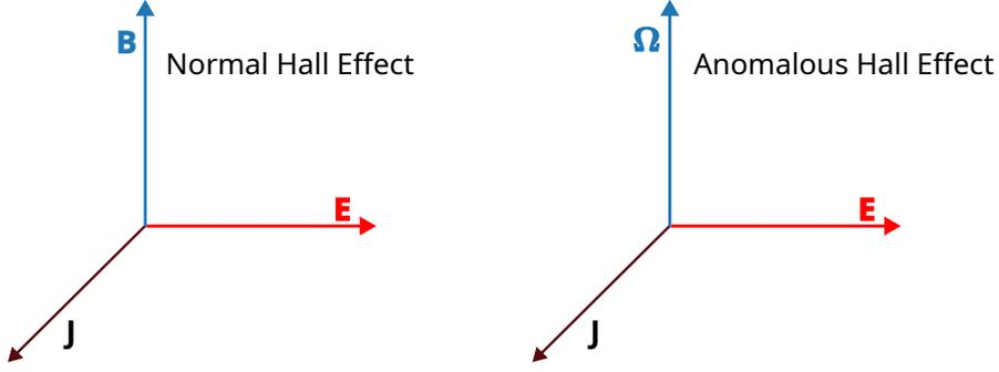
Figure 2.9: Left panel: Orthogonal electric and magnetic fields result in perpendicular electric current in normal Hall effect. Right panel: the role of the magnetic field is replaced by  $\Omega$  (“pseudo-magnetic field”) in the anomalous Hall effect.
