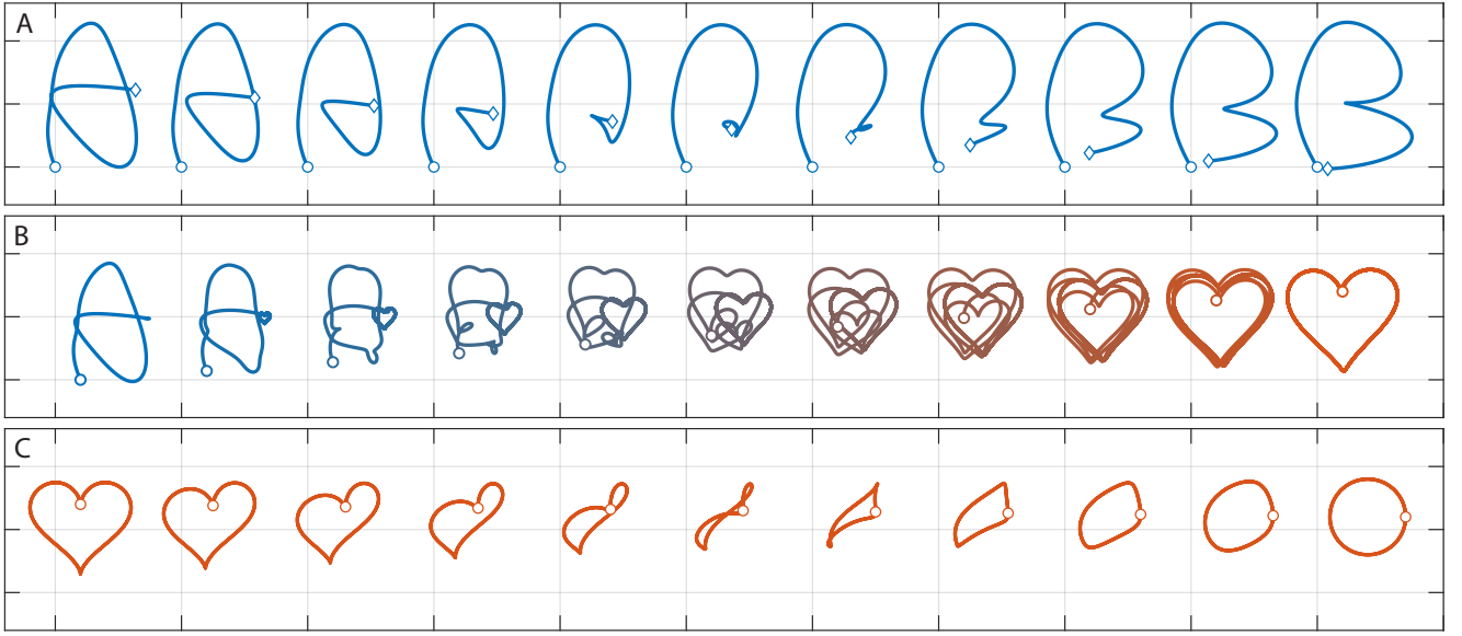
Fig. 2. Parallel combination of both discrete and rhythmic DMPs. (A) Parallel combination of discrete DMPs. For the combination, primitive inputs to generate the letters A and B were used. (B) Parallel combination of discrete and rhythmic DMPs. For the combination, primitive inputs to generate letter A (discrete) and heart (rhythmic) were used. (C) Parallel combination of rhythmic DMPs. For the combination, primitive inputs to generate heart and circle were used. For the 11 trajectories of each figure, the parameters used for parallel combination were \alpha_1 = [0.0, 0.1, \dots, 1.0] and \alpha_2 = 1 - \alpha_1 , ordered from left to right. DMP parameters used for Imitation Learning were identical to those in Figure 1. For all DMPs, the parameters for spatial scaling and rotation were \kappa_s = 1.0 , \mathbf{R} = \mathbb{I}_2 . For temporal scaling, \kappa_t = 1.0 was used for the trajectories in figure (A) and (C); for figure (B), \kappa_t = 0.25, 6.00 were used for letter A (discrete) and heart (rhythmic), respectively. For all figures, circle markers depict the start position for discrete and rhythmic DMPs; diamond markers depict the goal position of discrete DMP.
