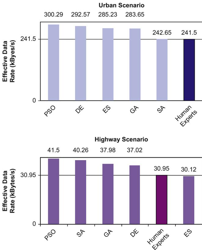
**Fig. 8.** Effective transmission data rates (throughput) (kBytes/s) achieved during the simulations of the final VDTP configurations in comparison with real car values given by human expert configurations (CARLINK).
