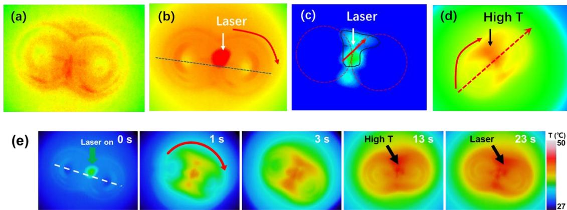
Figure 6. Thermal image of the clockwise rotation of two ferrofluid droplets. (a) thermal image without the laser, (b) the laser shines on the higher right of the FF, (c) the heat distribution at the beginning, and (d) (e)the heat distribution during rotation at the end.
