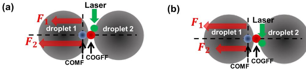
Figure 4. Rotation analysis diagram of the rotating motion of two ferrofluid droplets. (a) Horizontal clockwise rotation of the force diagram. (b) Horizontal clockwise rotation of the force diagram.
