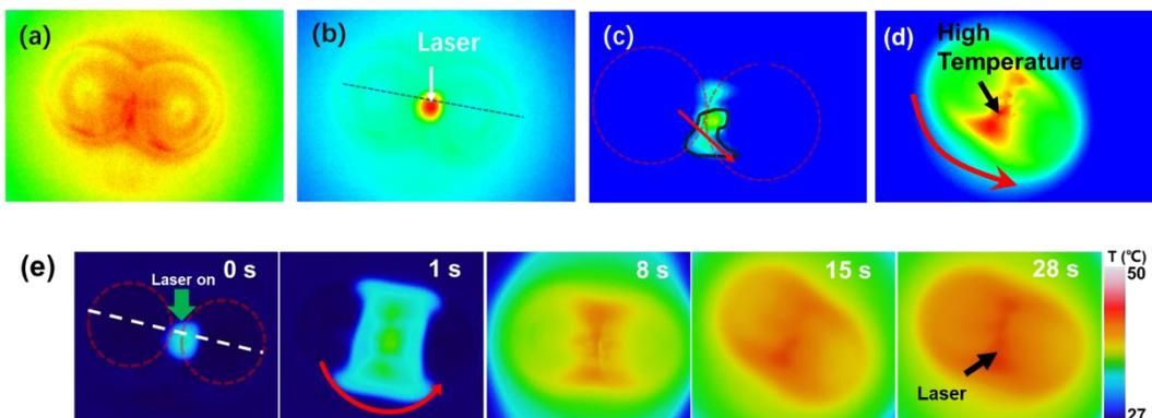
Figure 5. Thermal image of the Counterclockwise rotation of two ferrofluid droplets. (a) thermal image without the laser, (b) the laser shines on the lower right of the FF, (c) the heat distribution at the beginning, and (d) (e) is the heat distribution during rotation.
