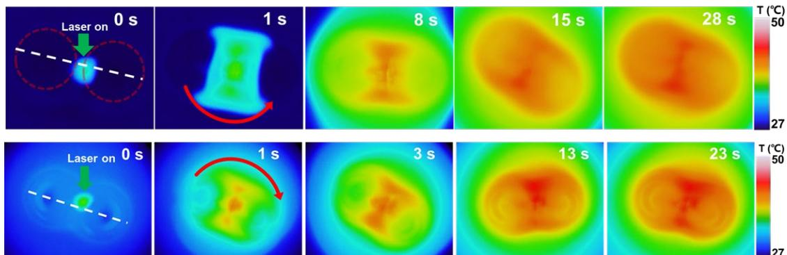
**Thermal Images of Rotating Ferrofluid**
