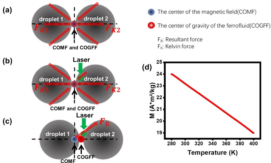
Figure 3. Schematic diagram of horizontal migration principle of laser-driven
