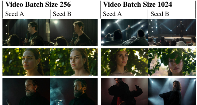
Figure 9. A large batch size prevents mode collapse. A small batch size has mode-collapsed across prompts and seeds.
