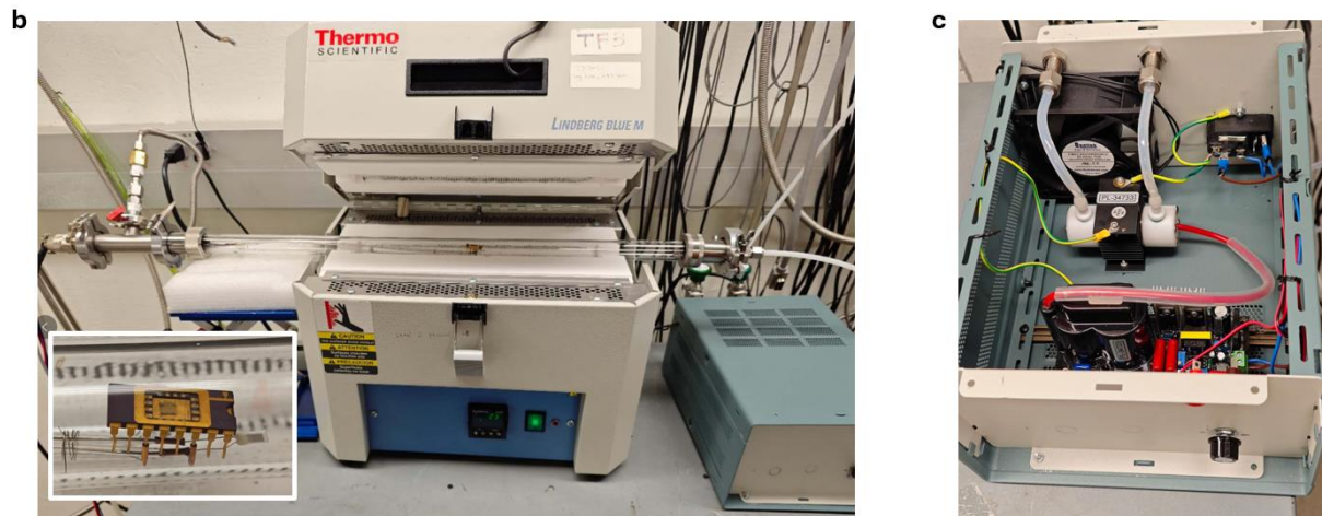
Extended Data Fig. 2 | Bespoke ozone annealing setup with in situ electrical transport. a , Schematic of the ozone annealing setup. b , Photograph of the setup, with an inset showing a film in the chip carrier inside the quartz tube. To the right of the chip carrier, a PT1000 sensor is positioned to measure the temperature at the chip carrier. c , Interior of the ozone generator, consisting of a tunable high voltage module (front), an ozone quartz generator with inlet and outlet (centre), and a cooling fan (back). A power meter is connected to the high voltage module to monitor the power which regulates w(\text{O}_3) .
