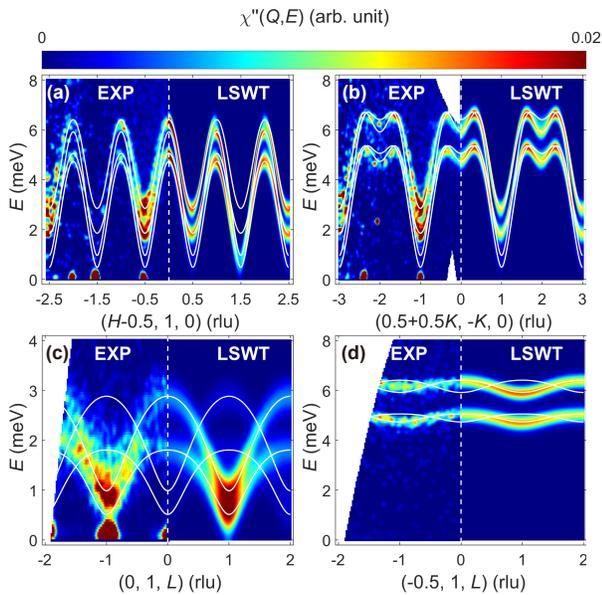
FIG. 3. Comparisons between the measured (EXP, left side in each panel) and calculated magnetic excitation spectra using the linear-spin-wave theory (LSWT, right). Directions of the dispersions are depicted in Fig. 2(b) and (c). The experimental data were collected at 7 K. Solid curves denote the calculated magnon dispersions.
