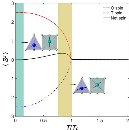
FIG. 4. Calculated temperature dependence of the  $z$ -components of the octahedral, tetrahedral, and net spin moments using self-consistent mean-field theory. The insets are schematic diagrams which show the relative tilting of octahedral and tetrahedral spins from the  $c$ -axis. Note that the tilting angles just below the transition temperature are arbitrary and only to emphasize that the different tilting angles will result in a net magnetization along the  $c$ -axis.
