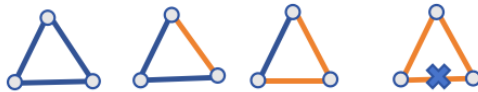
FIG. SM-2. The blue lines represent ferromagnetic interactions, while the yellow lines represent antiferromagnetic interactions. The fourth scenario depicted in the diagram does not exist.
