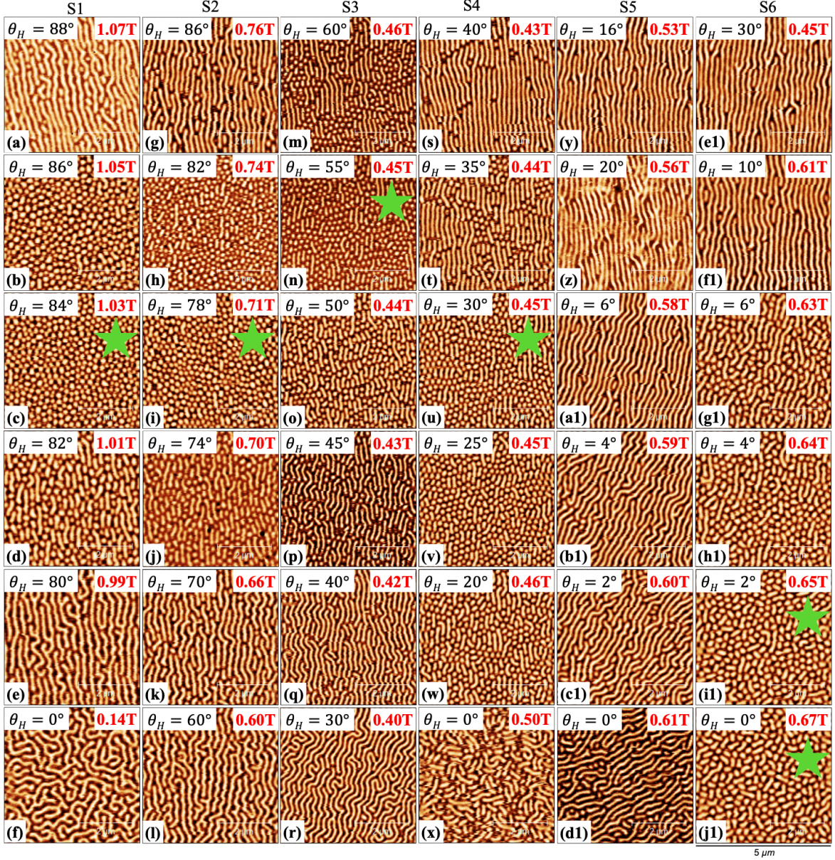
Figure 2: (a-f), (g-l), (m-r), (s-x), (y-d1) and (e1-j1) represent the angle-dependent MFM for the Co thicknesses of 8 Å, 10 Å, 12 Å, 16 Å, 20 Å, and 24 Å, respectively, at remanence after applying different DC saturation fields under different angles and reduction to zero according to the protocol described in the main text. All MFM images have the same area-of-view equal to 25 \mu\text{m}^2 .
