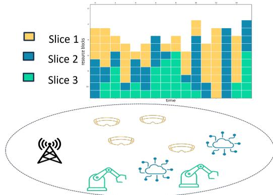
Fig. 1. Illustration of a RAN slicing system
